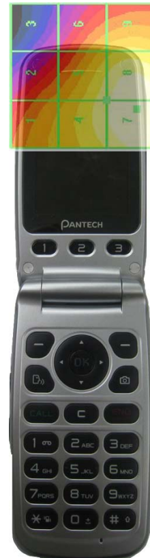
GSM H-Field WD Scan overlay
