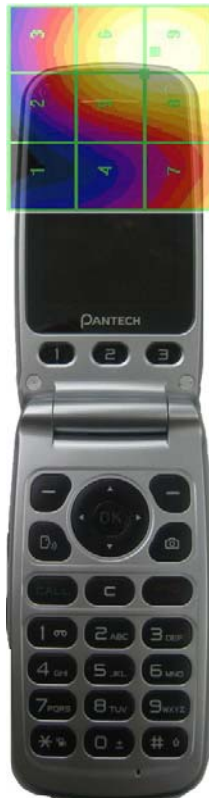
GSM E-Field WD Scan overlay
