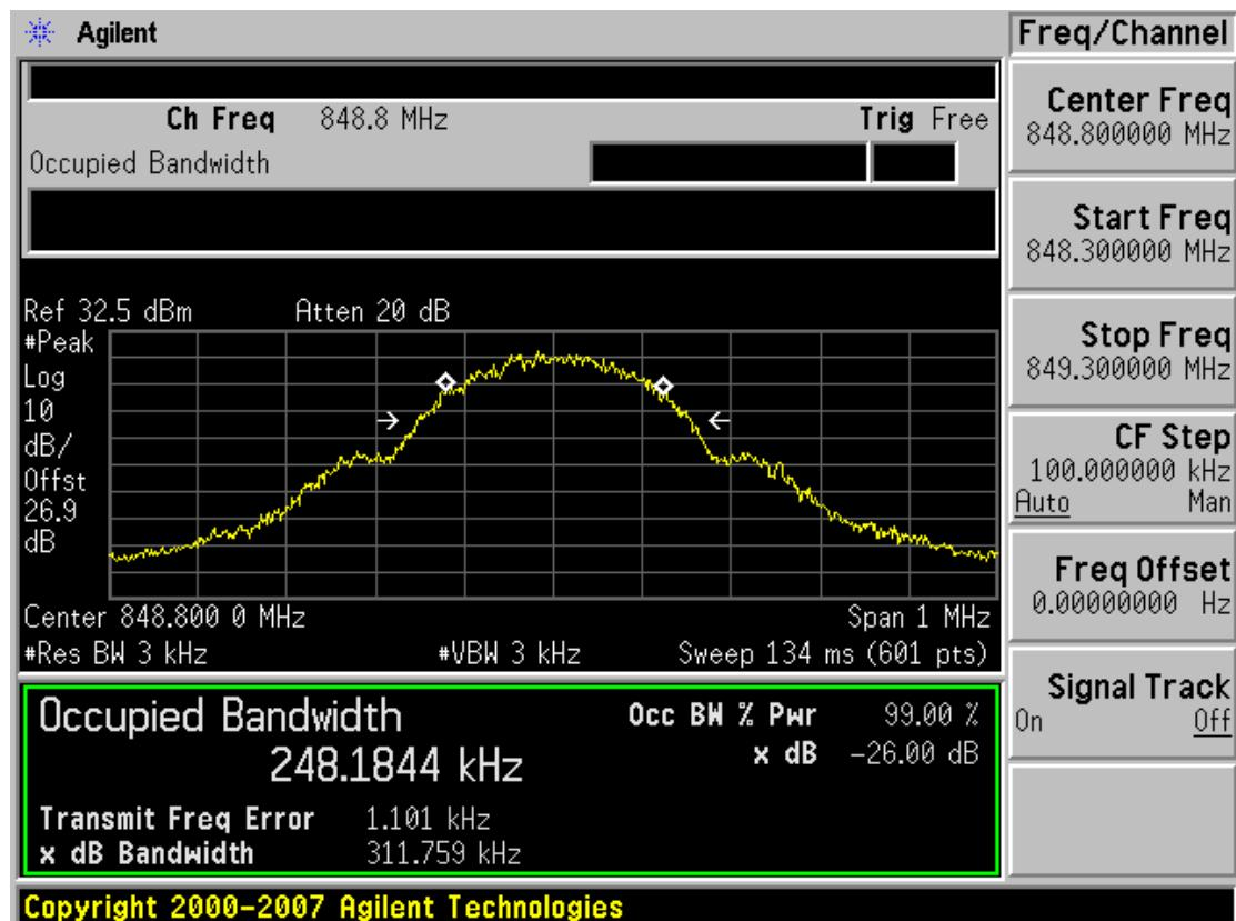
■ GSM850 EDGE (251 CH.) Occupied Bandwidth
