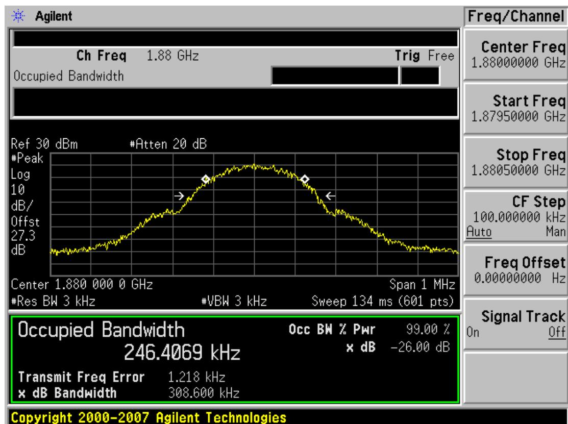
■ GSM1900 MODE (810 CH.) Occupied Bandwidth
