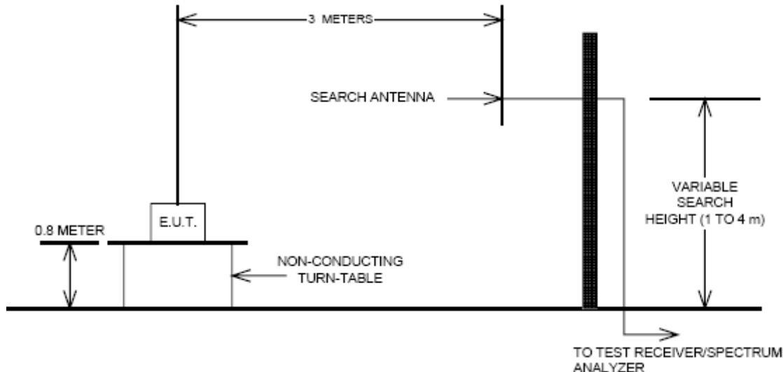
The measurement facilities used for this test have been documented in previous filings with the commission pursuant to section § 2.948. The Fully-anechoic chamber meets requirements in ANSI C63.4 –2003. A mast capable of lifting the receiving antenna from a height of one to four meters is used together with a rotatable platform mounted at three from the antenna mast.
