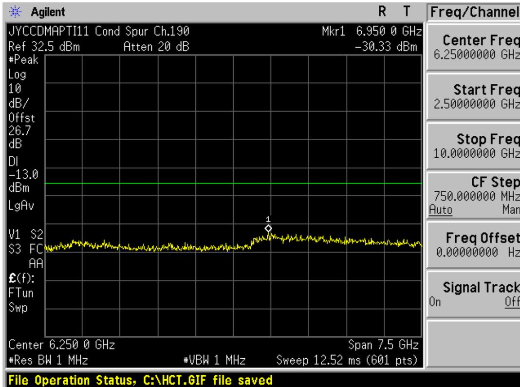
■ GSM850 MODE (251 CH.) Conducted Spurious Emissions1
