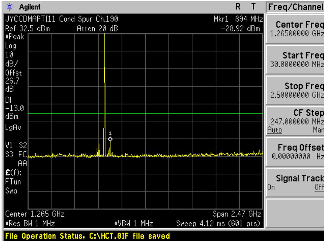
■ GSM850 MODE (190 CH.) Conducted Spurious Emissions2
