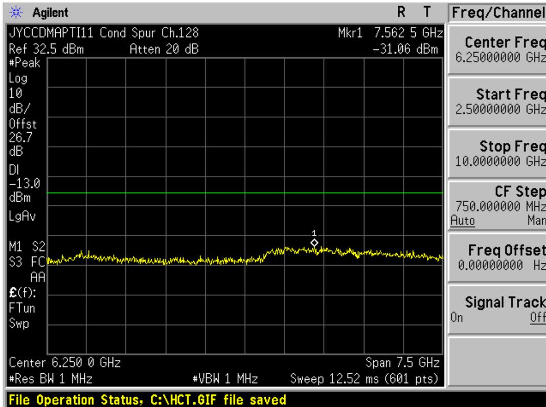
■ GSM850 MODE (190 CH.) Conducted Spurious Emissions1
