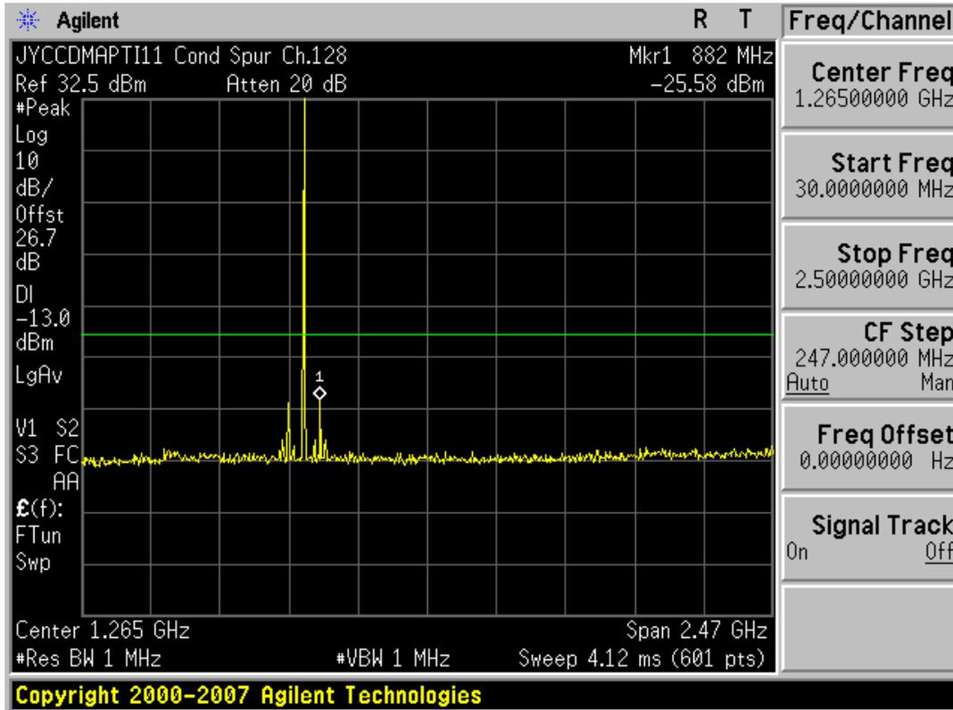
■ GSM850 MODE (128 CH.) Conducted Spurious Emissions2
