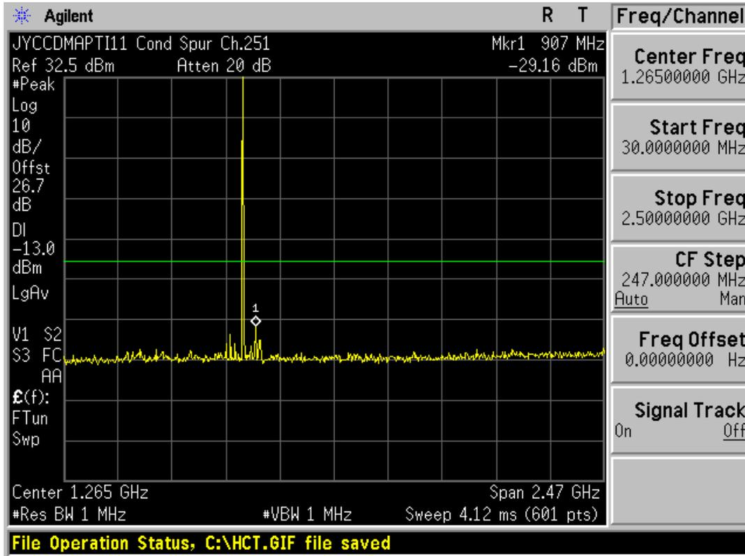
■ GSM850 MODE (251 CH.) Conducted Spurious Emissions2
