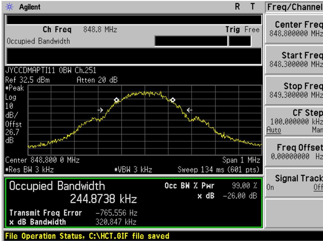
■ GSM1900 MODE (512 CH.) Occupied Bandwidth
