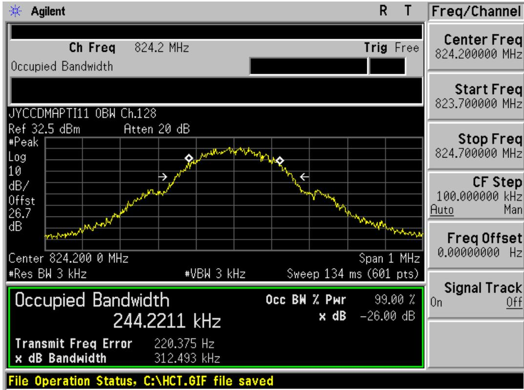
■ GSM850 MODE (190 CH.) Occupied Bandwidth
