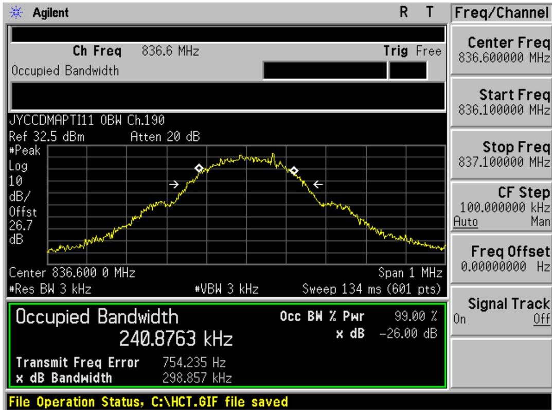
■ GSM850 MODE (251 CH.) Occupied Bandwidth
