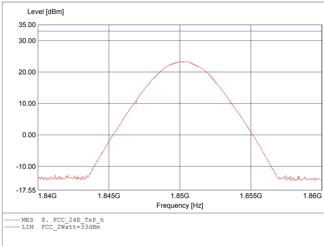
**Equivalent Isotropically Radiated Power
