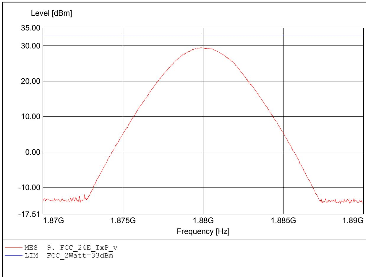
**Equivalent Isotropically Radiated Power
