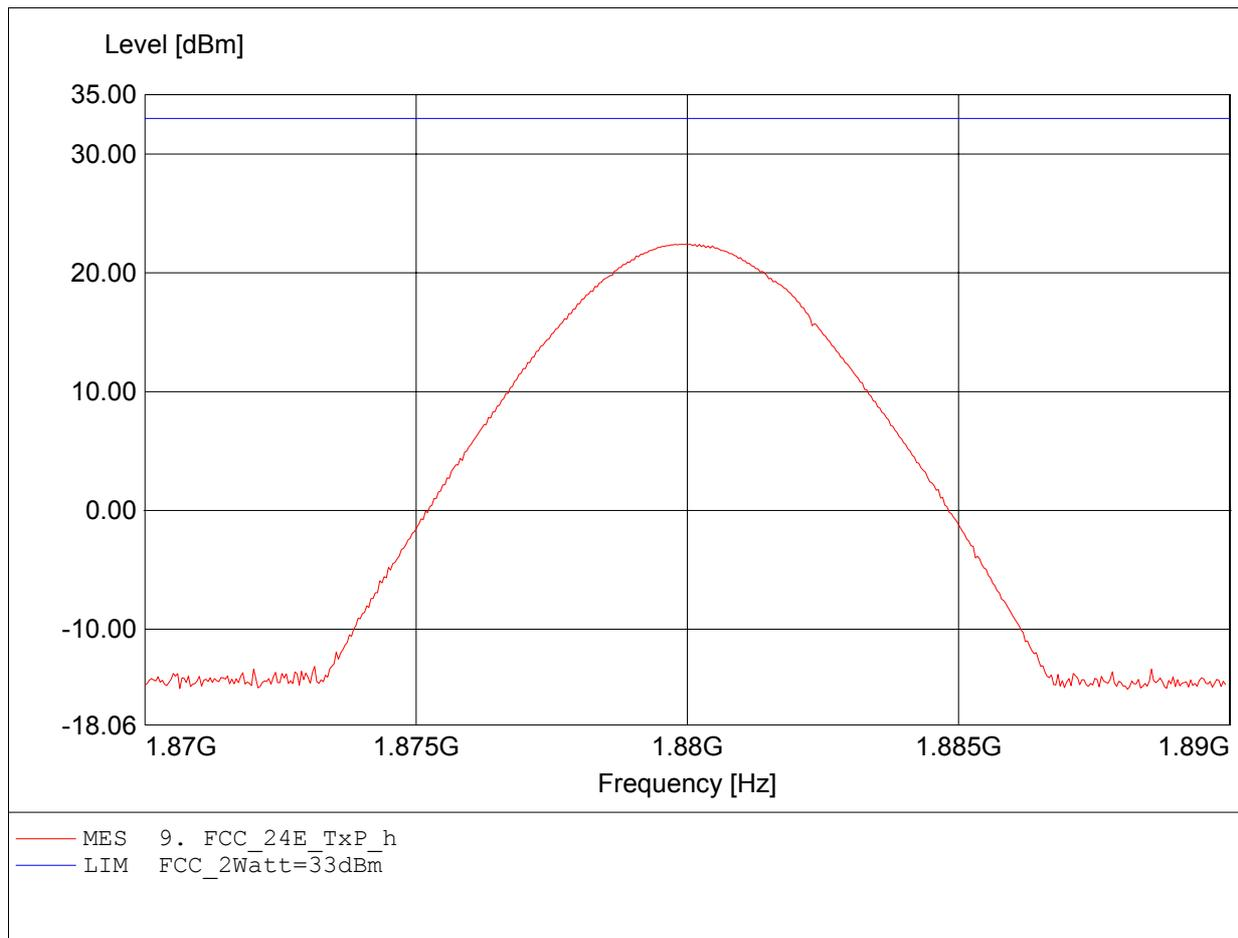
**Equivalent Isotropically Radiated Power
