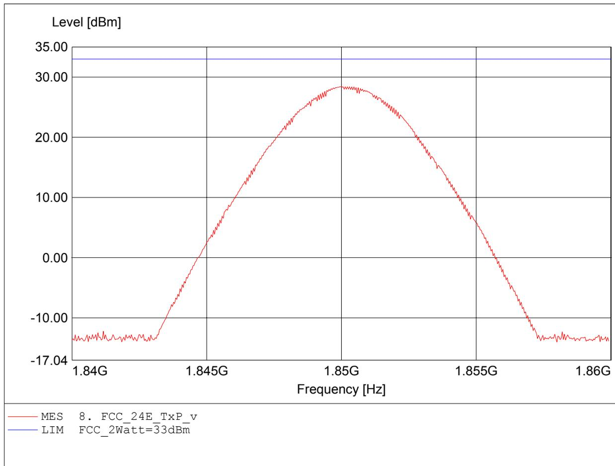
**Equivalent Isotropically Radiated Power
