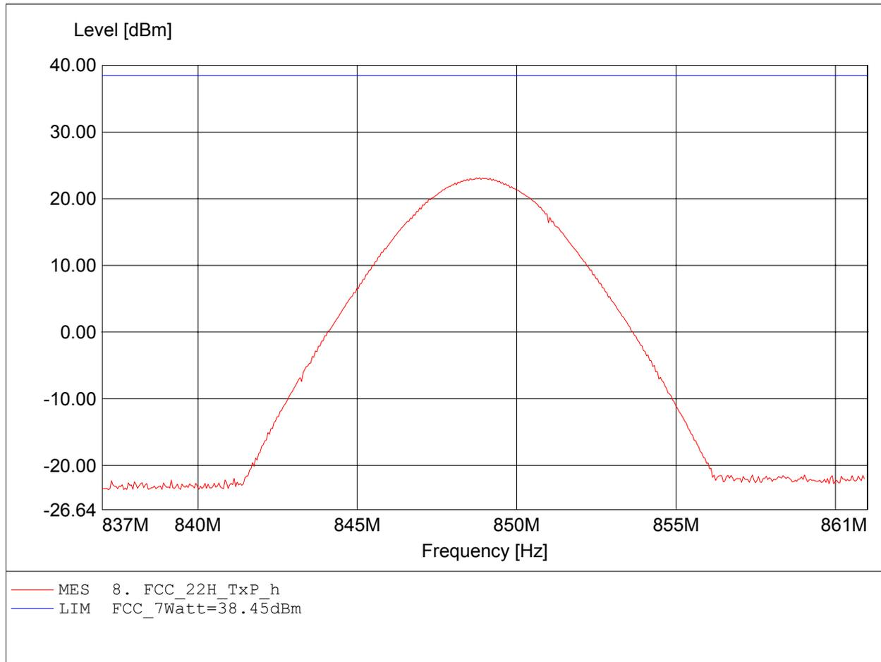
**Equivalent Isotropically Radiated Power
