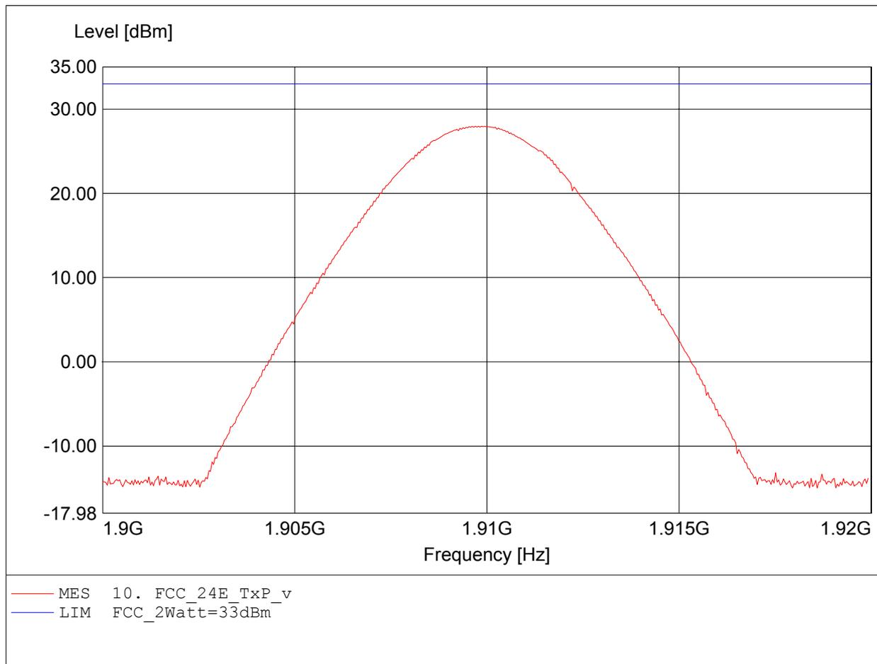
**Equivalent Isotropically Radiated Power
