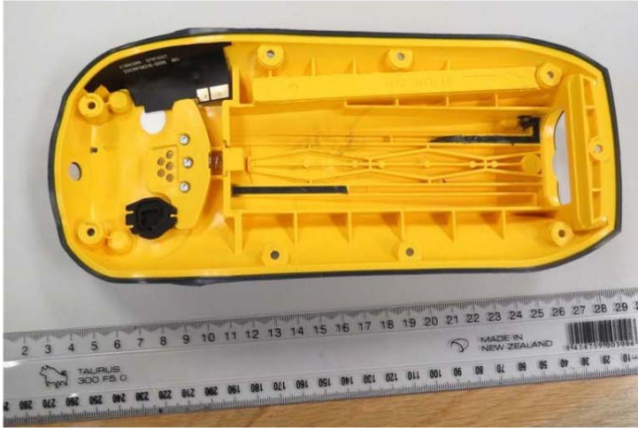
Lower half of enclosure showing Cellular Antenna
