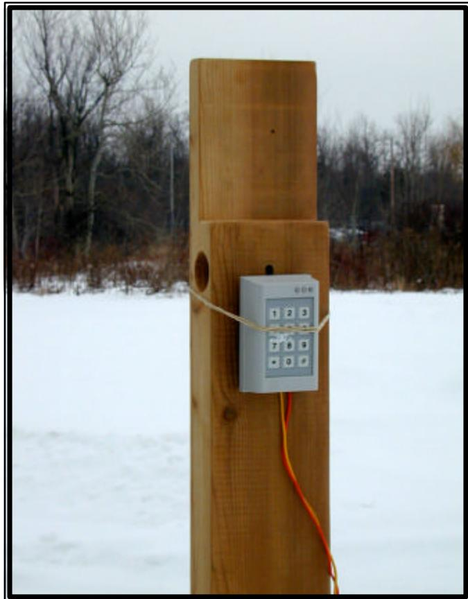
**Section 4. Frequency Stability****Para. No.: 15.225****Test Performed By:** Russell Grant**Date of Test:** January 9, 2002**Minimum Standard:** 0.01%, 100 ppm, 1356 Hz**Test Results:** Complies.**Measurement Data:** STV: 12 VDC
