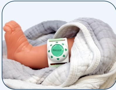
TotTags work with the GuardRFID AllGuard® software with TotGuard® support to provide real-time location services. The tag's built-in dual tamper detection capability allows the software to generate an alarm if the tag is tampered or removed from the infant, while minimizing false alarms caused by normal infant care. The AllGuard software can be configured to control doors to speed newborns to scheduled medical examinations or protect babies from suspicious activity.
