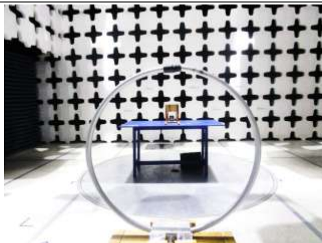
Radiated Emissions (<30MHz) – Front View 0 degree
