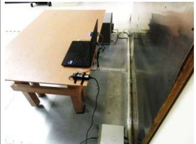
AC Line Conducted Emissions– Rear View
