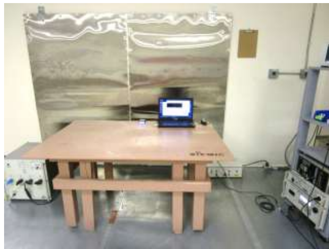
AC Line Conducted Emissions– Front View
