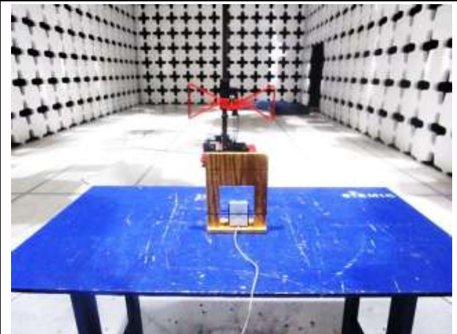
Radiated Emissions (<1GHz) – Rear View
