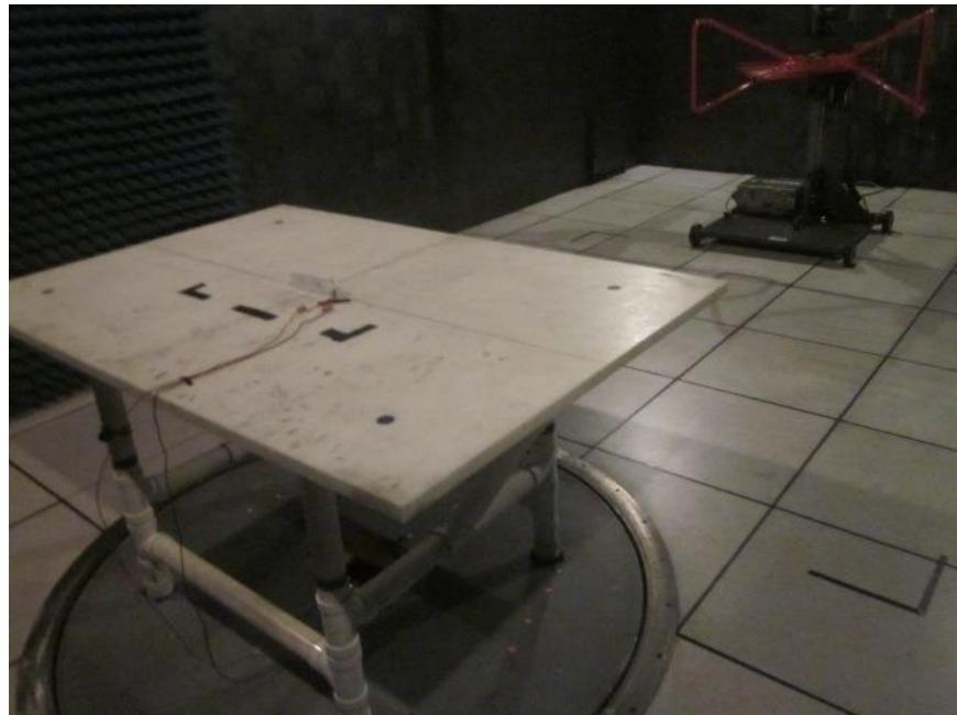
**1 GHz - 18 GHz Radiated Emission**
