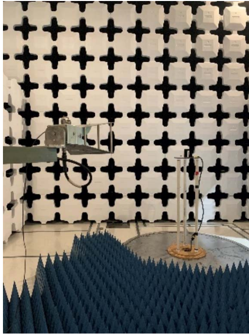
Figure 53: Cabinet Radiated emission setup 1-18GHz
