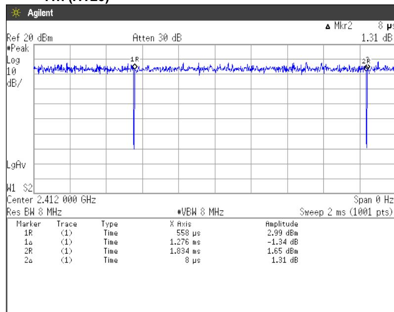
$$\text{Duty Cycle} = \text{Ton} / (\text{Ton} + \text{Toff}) = 1276[\mu\text{s}] / (1276[\mu\text{s}] + 8[\mu\text{s}]) = 99.38\%]$$
