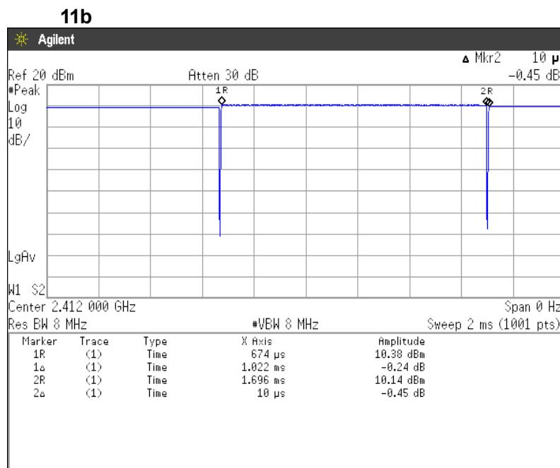
$$\text{Duty Cycle} = \text{Ton} / (\text{Ton} + \text{Toff}) = 1022[\mu\text{s}] / (1022[\mu\text{s}] + 10[\mu\text{s}]) = 99.03\%]$$
