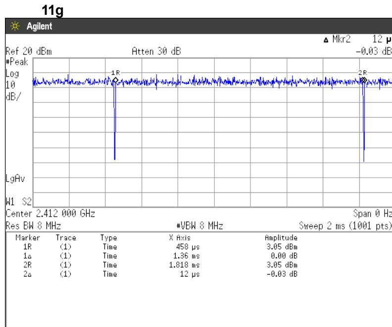
$$\text{Duty Cycle} = \text{Ton} / (\text{Ton} + \text{Toff}) = 1360[\mu\text{s}] / (1360[\mu\text{s}] + 12[\mu\text{s}]) = 99.13\%$$
