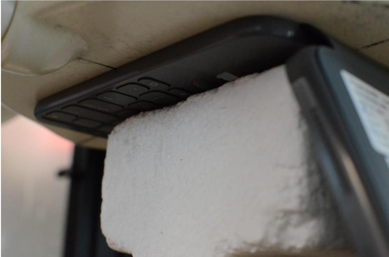
**SAR Test Setup Photo 1: Body, Keyboard Accessory Case, Back Side, 0 mm**
