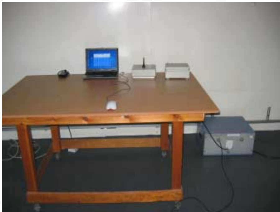
Photograph No.5 Conducted emissions measurement setup
