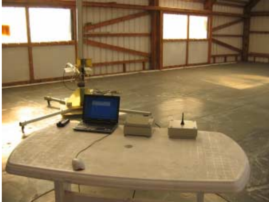
Photograph No.4 Radiated emissions measurement setup close view
