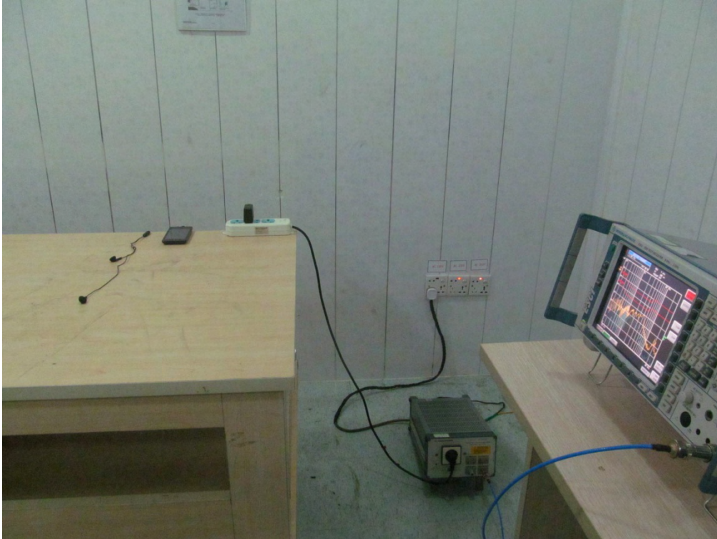
FCC LINE CONDUCTED EMISSION TEST SETUP
