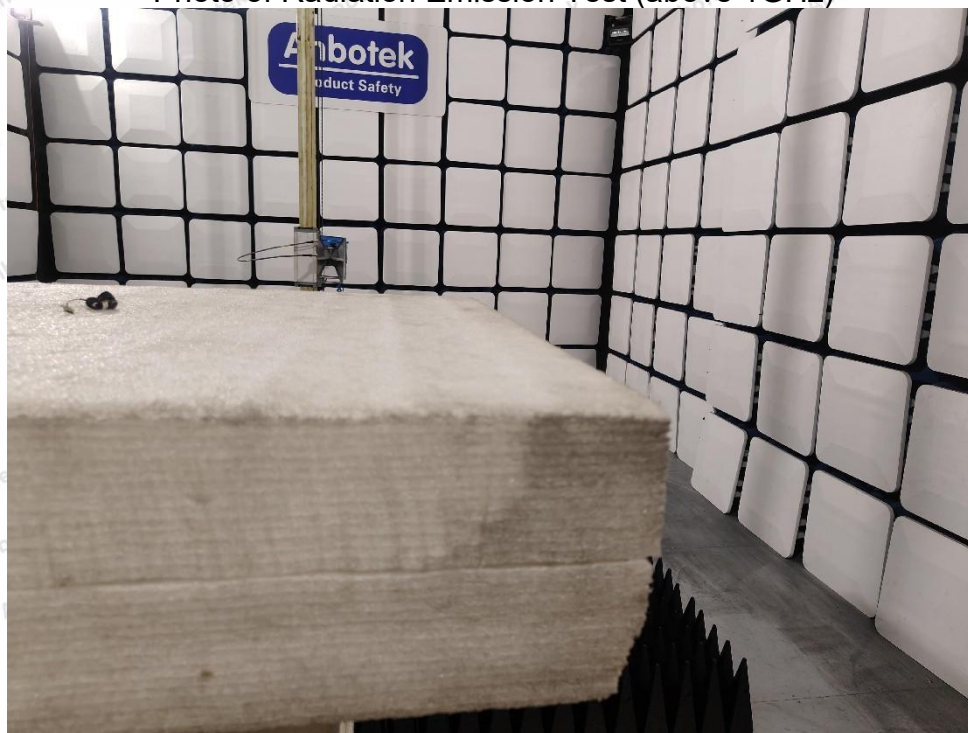
Photo of Radiation Emission Test (above 1GHz)
