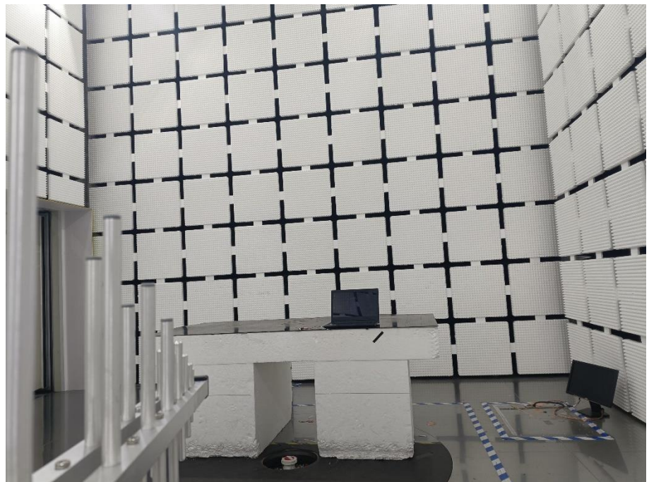
Radiation Emission Test Setup (30MHz to 1GHz)
