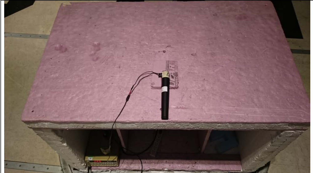
FIELD STRENGTH SPURIOUS EMISSIONS TABLE SETUP
