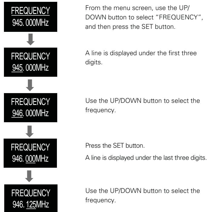
From the menu screen, use the UP/DOWN button to select "FREQUENCY", and then press the SET button.
