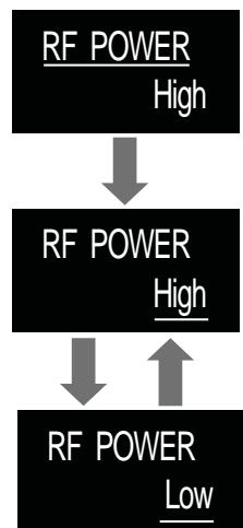
From the menu screen, use the UP/DOWN button to select "RF POWER", and then press the SET button.
