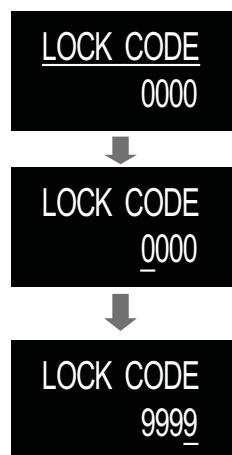
From the menu screen, use the UP/DOWN button to select "LOCK CODE", and then press the SET button.
