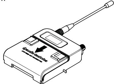
3. Then, open the battery cover as shown in the diagram.
