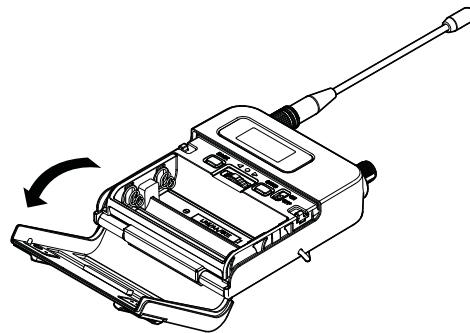
4. Insert the batteries correctly according to the plus (+) and minus (-) marks indicated on the product.
