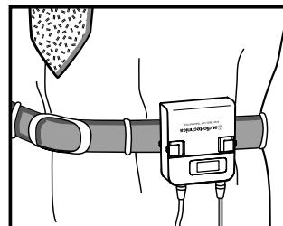
Pull both sides of the clip firmly to the outside to remove the clip from the product.
