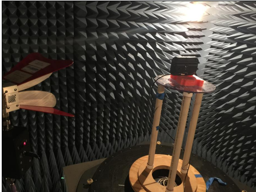
Photograph 2. Radiated Emissions, Test Setup, Above 1 GHz
