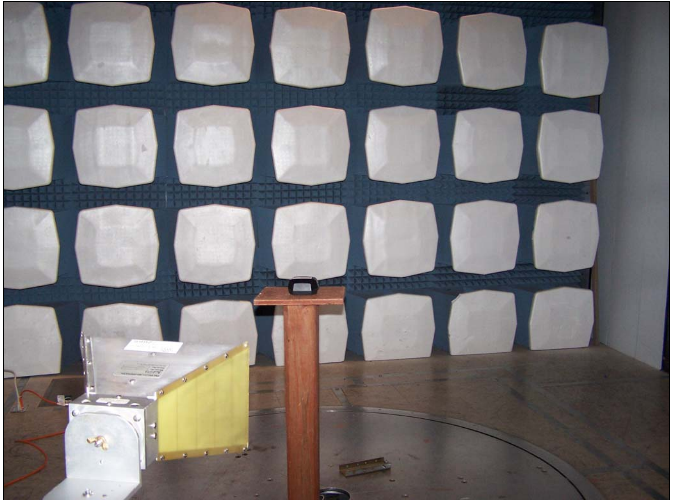
Photograph 4. Radiated Emission Test Setup - above 1 GHz
