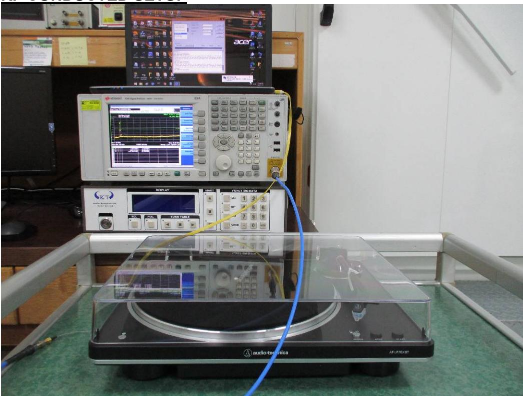
**CONDUCTED EMISSION MEASUREMENT SETUP****MODE: NORMAL OPERATION**
