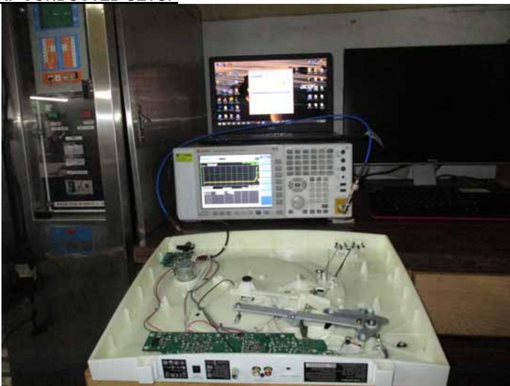
**CONDUCTED EMISSION MEASUREMENT SETUP****MODE: NORMAL OPERATION**
