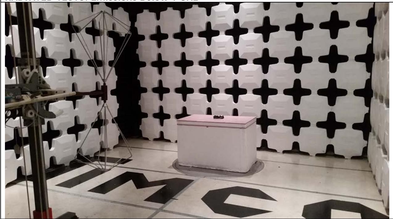
**RADIATED TESTS: Emissions Above 1 GHz**
