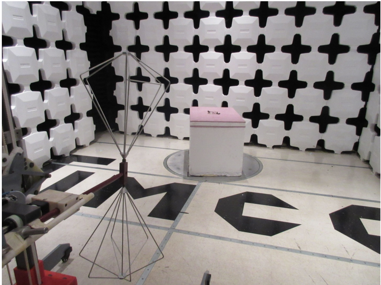
RADIATED EMISSIONS TEST SET UP PHOTO BELOW 1GHZ
