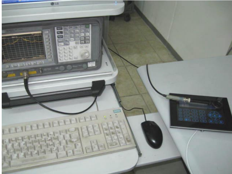
Photograph No.5 Occupied bandwidth measurement setup
