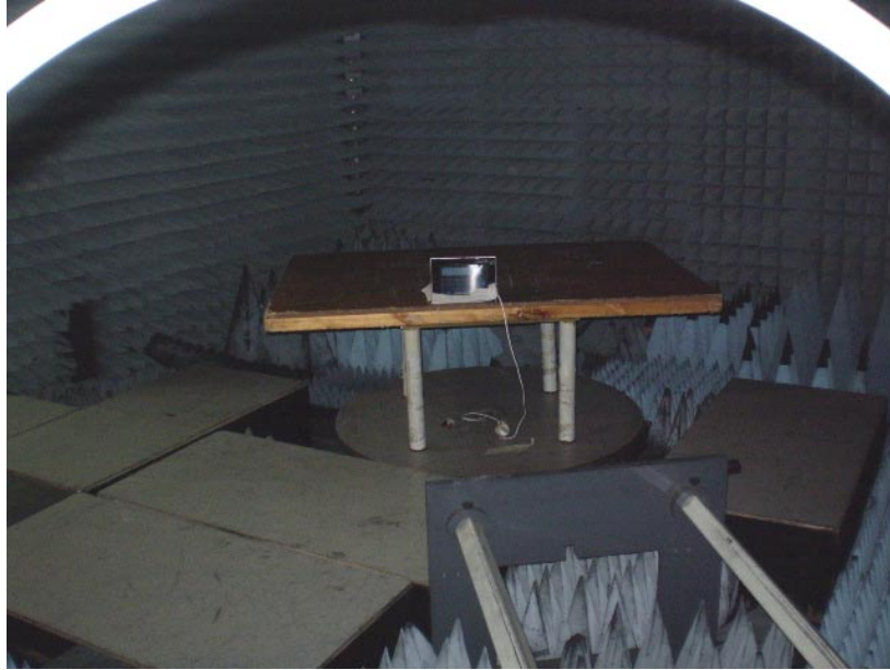
Photograph No.2 In-band and spurious emissions field strength measurement setup below 30 MHz in the anechoic chamber
