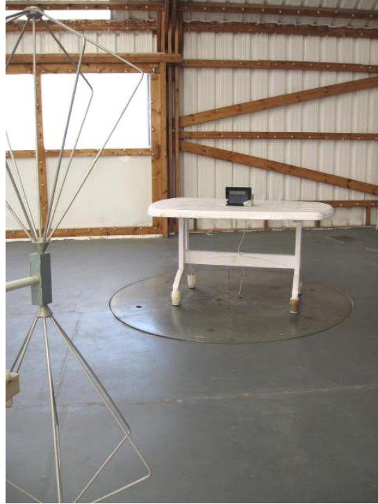
Photograph No.4 Spurious emissions measurement setup from 30 MHz to 1000 MHz at the OATS
