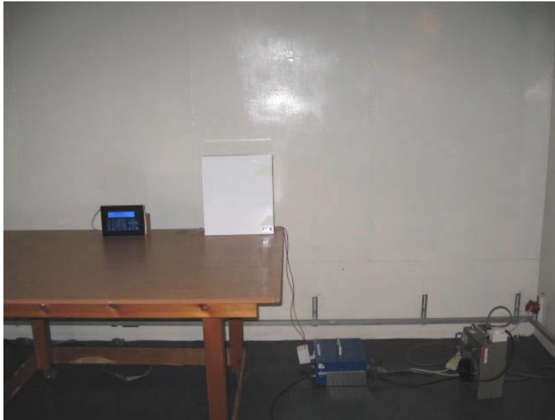
Photograph No.7 Setup for conducted emission measurements at the EUT power port
