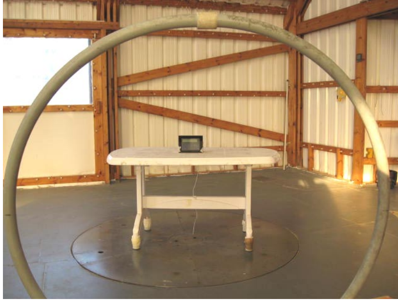
Photograph No.1 In-band emissions field strength measurement setup at the OATS
