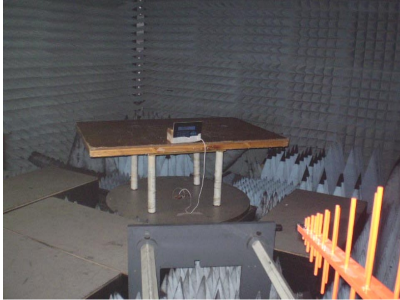
Photograph No.3 Spurious emission measurement test setup from 30 MHz to 1000 MHz in the anechoic chamber
