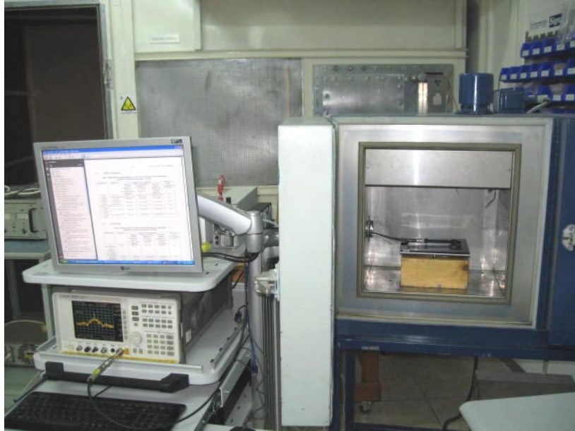
Photograph No.6 Frequency stability measurements setup
