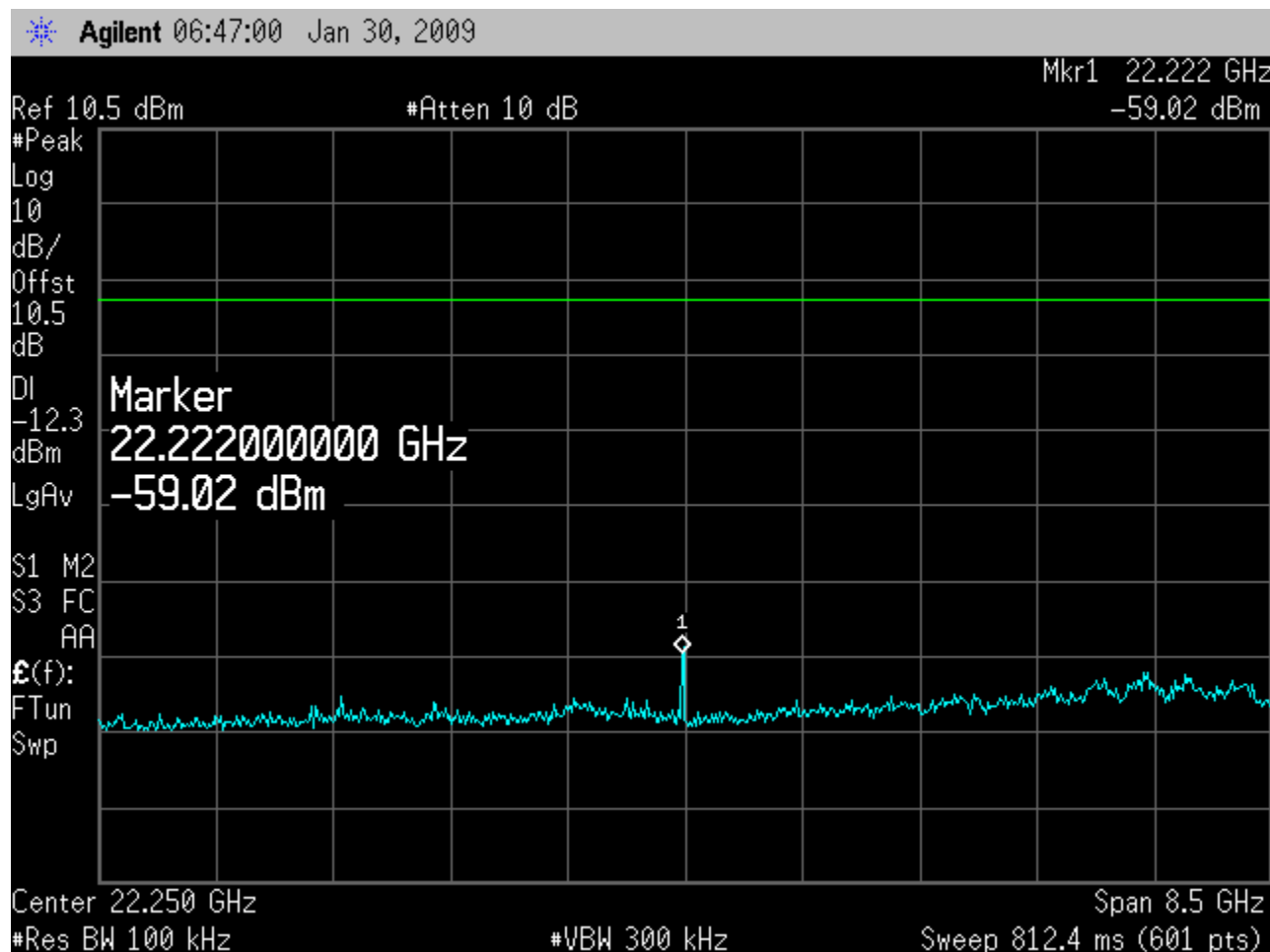
Plots from 18 to 26.5GHz (Peak) High Channel, Display Line (-12.33 dBm) is the line 30dB below the highest inband emission.
