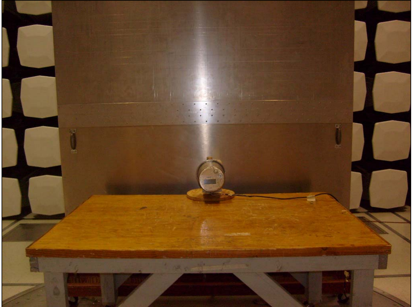
Photograph 1. Conducted Emissions, Test Setup
