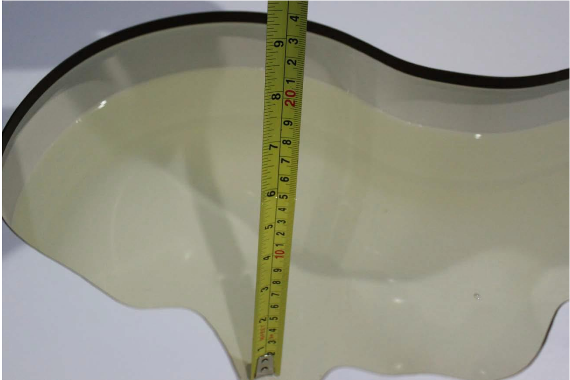
Picture 7-3: Liquid depth in the Head Phantom (5GHz)
