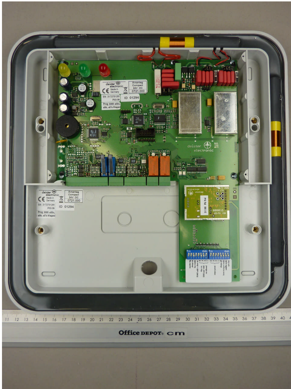
111945_b.JPG: Amantag Compact, internal view, internal cover removed
