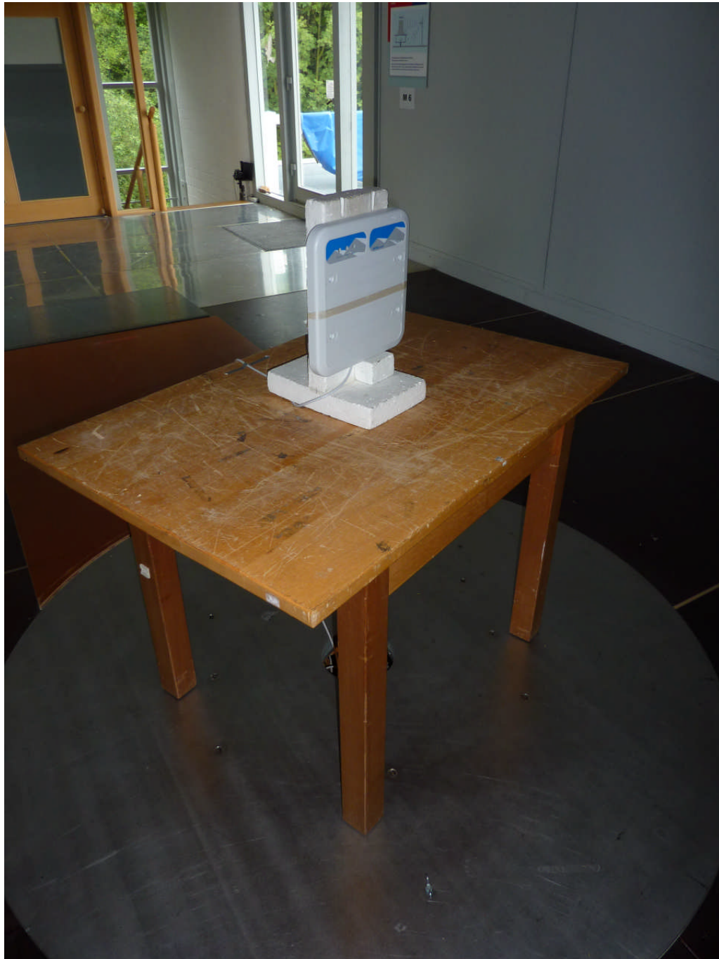
111945_4.JPG: Amantag Compact, test setup open area test site
