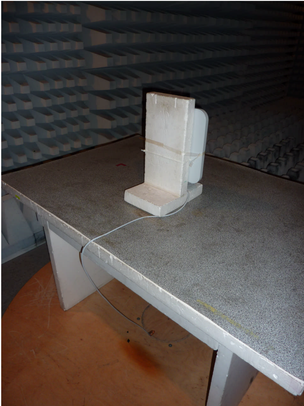
111945_3.JPG: Amantag Compact, test setup fully anechoic chamber
