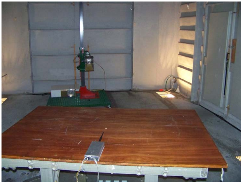
Radiated Emissions, Horizontal Polarity, Test Distance, Double Ridged Guide Antenna
