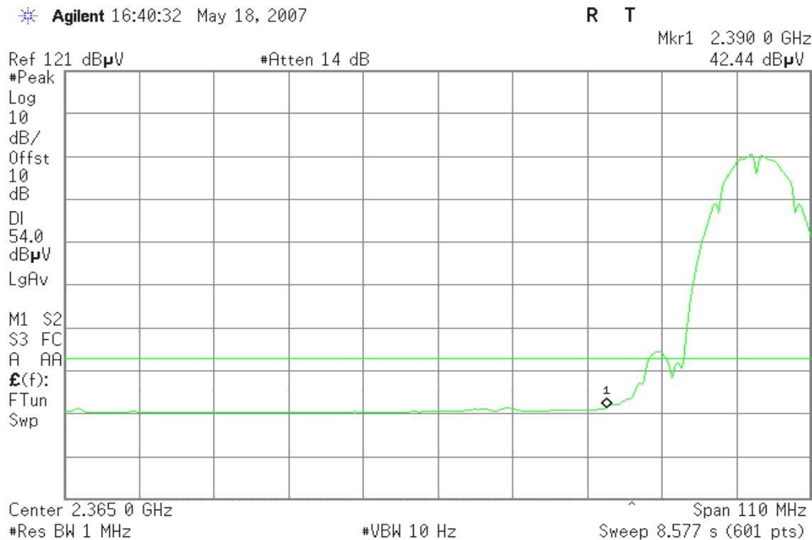
**Detector mode: Peak****Polarity: Horizontal**
