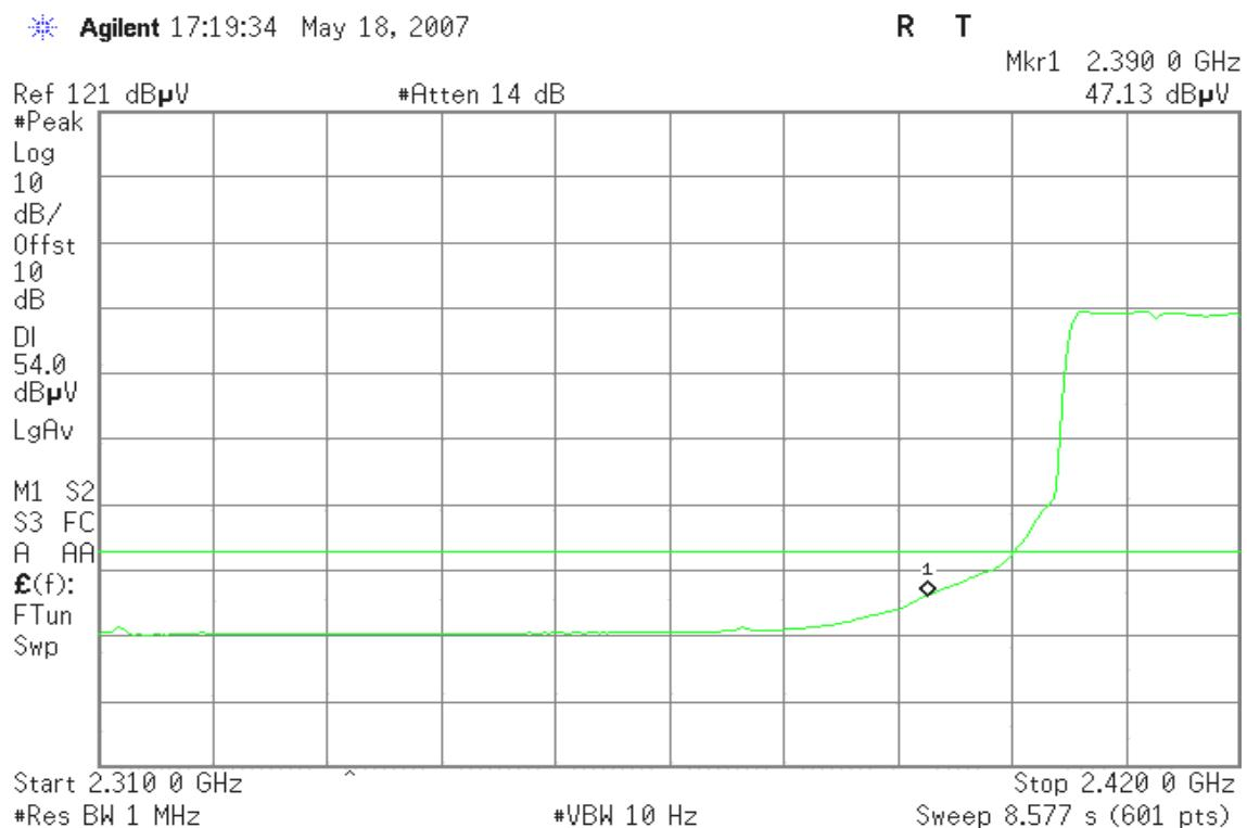
**Band Edges (IEEE 802.11g mode / CH High)****Detector mode: Peak****Polarity: Vertical**
