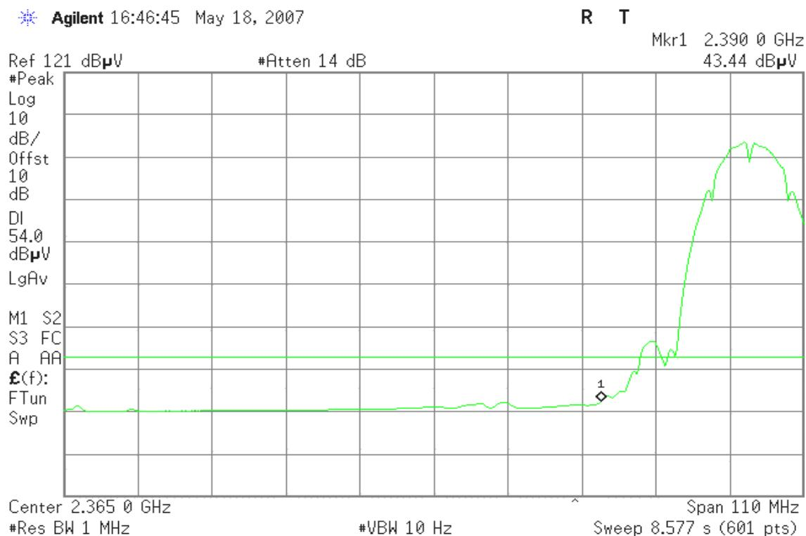
**Band Edges (IEEE 802.11b mode / CH High)****Detector mode: Peak****Polarity: Vertical**
