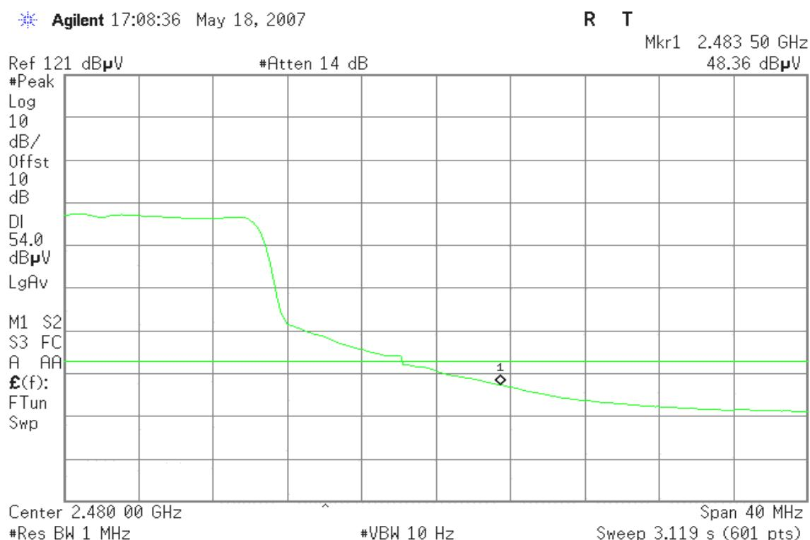
**Detector mode: Peak****Polarity: Horizontal**
