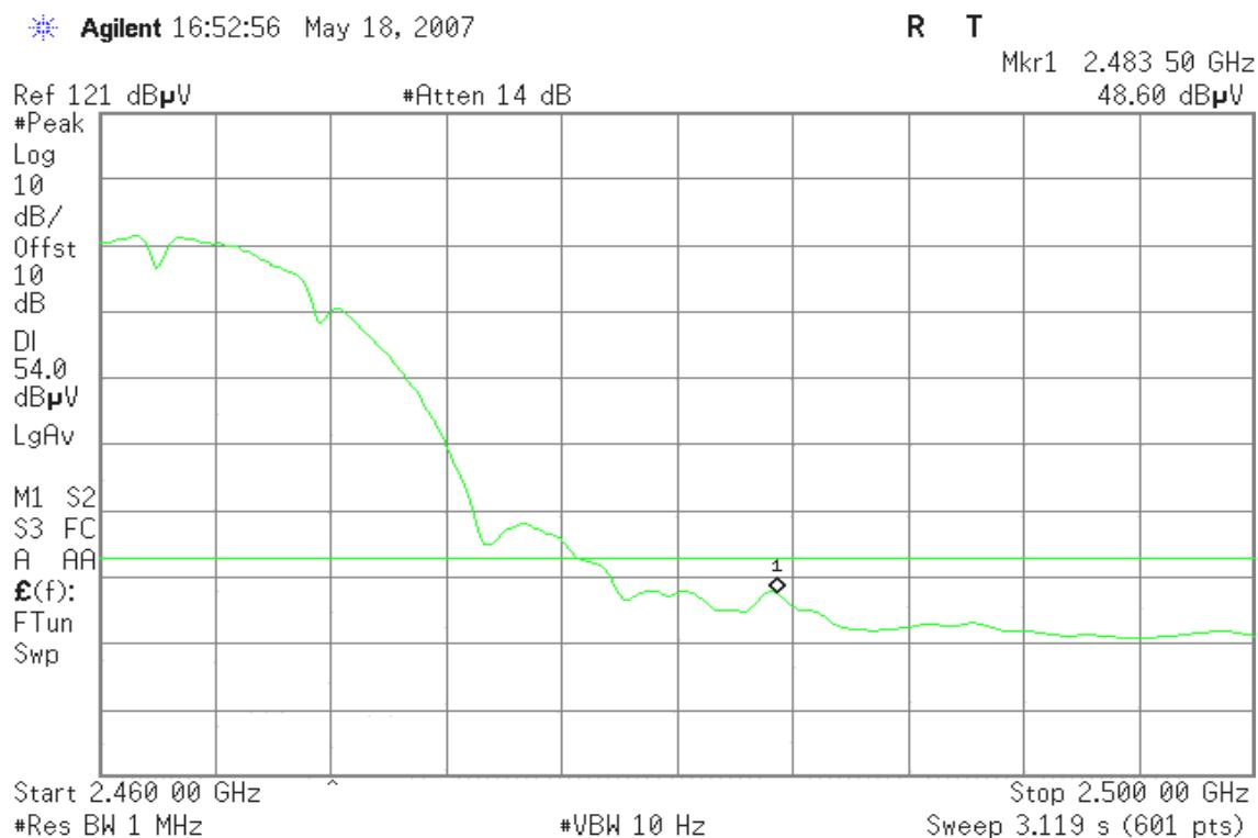
**Band Edges (IEEE 802.11g mode / CH Low)****Detector mode: Peak****Polarity: Vertical**
