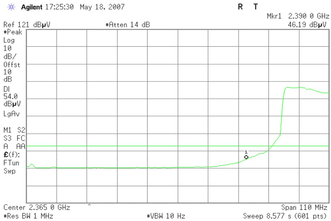
**Detector mode: Peak****Polarity: Horizontal**
