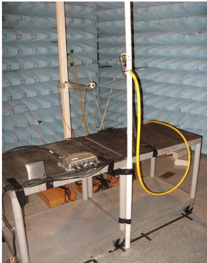
Immunity to Radio Frequency Electromagnetic Field (Enclosure Port)
