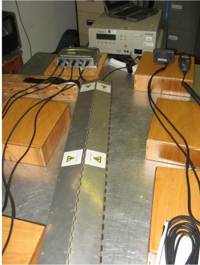
Immunity to Fast Transient Bursts Common Mode (Signal, Control and Telecommunications Port)
