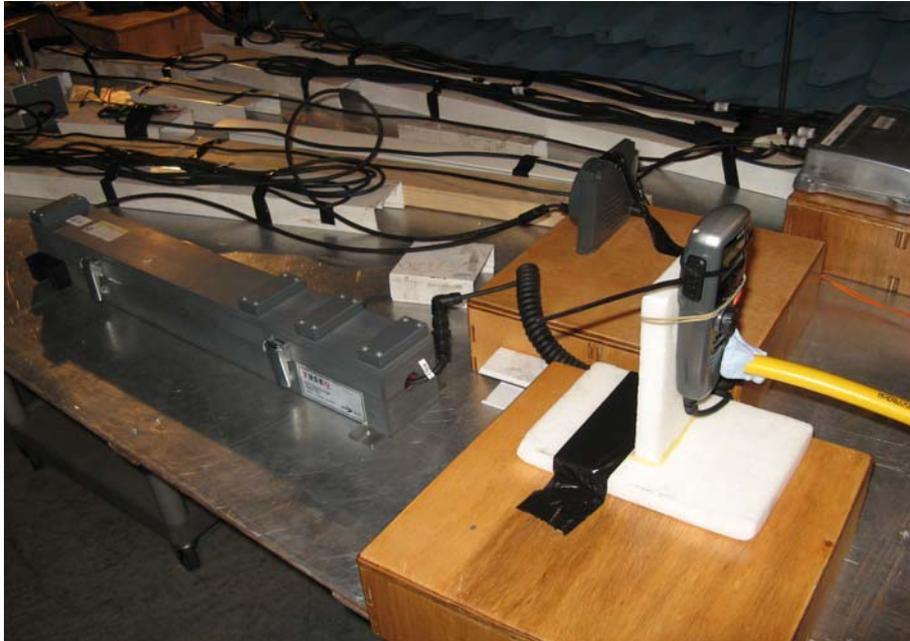
Immunity to Radio Frequency Common Mode (Signal, Control and Telecommunications Port)
