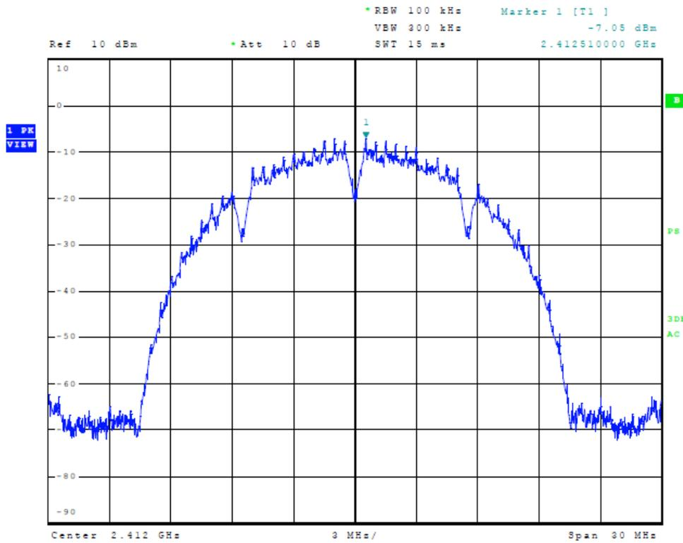
**Figure 13 Plot of Transmitter Peak Power Spectral Density (PKPSD) (802.11 b-mode)**
