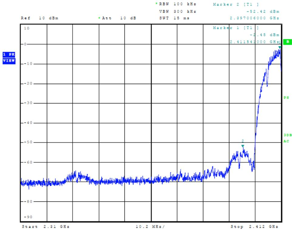
**Figure 7 Plot of Lower Band Edge (802.11 b-mode)**
