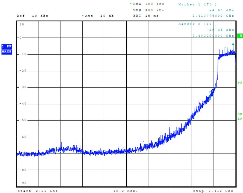
**Figure 8 Plot of Lower Band Edge (802.11 g-mode)**
