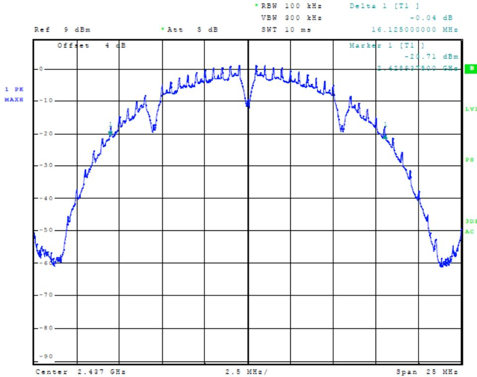
Figure 11 Plot of Transmitter Occupied Bandwidth (802.11 b-mode)
