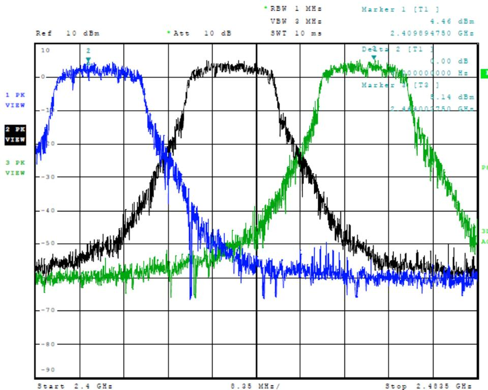
Figure 6 Plot of Transmitter Emissions in Operational Frequency (802.11 G Mode)
