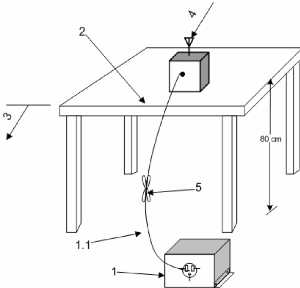
1. A LISN is optional for radiated measurements between 30 MHz to 1000 MHz, but not allowed for measurements below 30 MHz and above 1000 MHz. (See 6.4.3, 6.5.1, and 6.6.3.) If used, connect EUT to one LISN. Unused LISN measuring port connectors shall be terminated in 50Ω. LISN can be placed on top of, or immediately beneath, reference ground plane (see 6.2.2 and 6.2.3.1).
