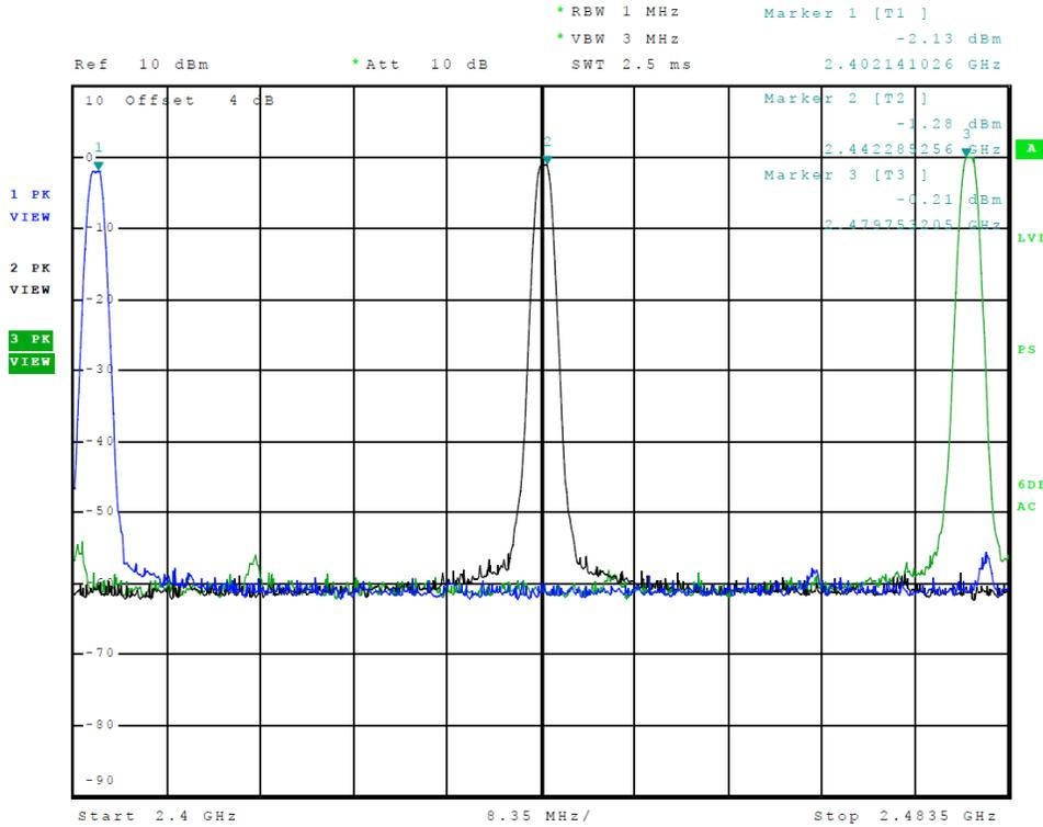
**Figure 3 Plot of Transmitter Emissions Operation in 2402-2480 MHz**
