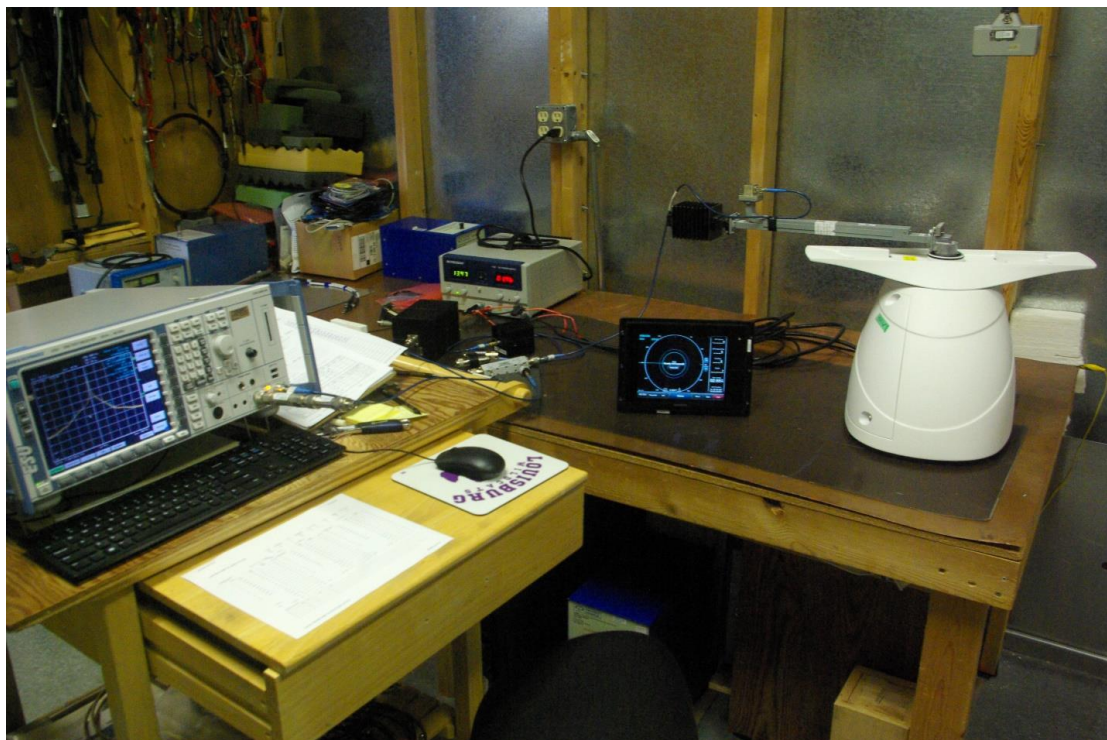
Antenna Port Conducted Emissions Test Setup
