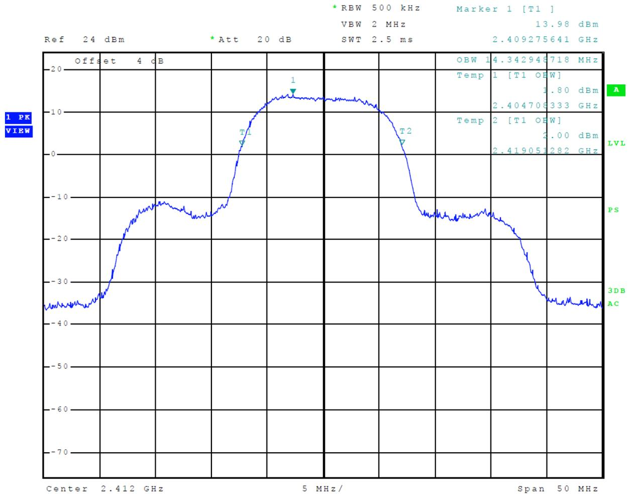
**Figure 14 Plot of 6-dB Occupied Bandwidth Mode 5 (DSSS)**
