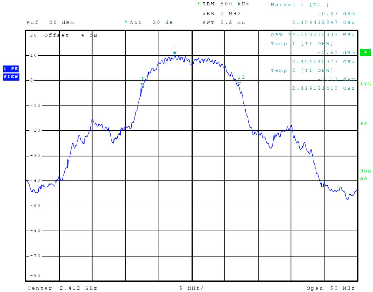
**Figure 15 Plot of 99% Occupied Bandwidth Mode 5 (DSSS)**
