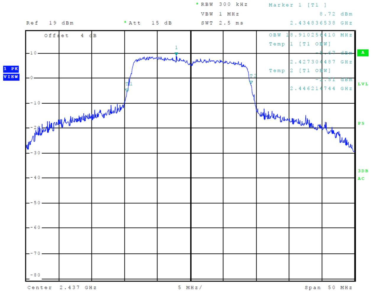
**Figure 19 Plot of 99% Occupied Bandwidth Mode 7 (MCS)**
