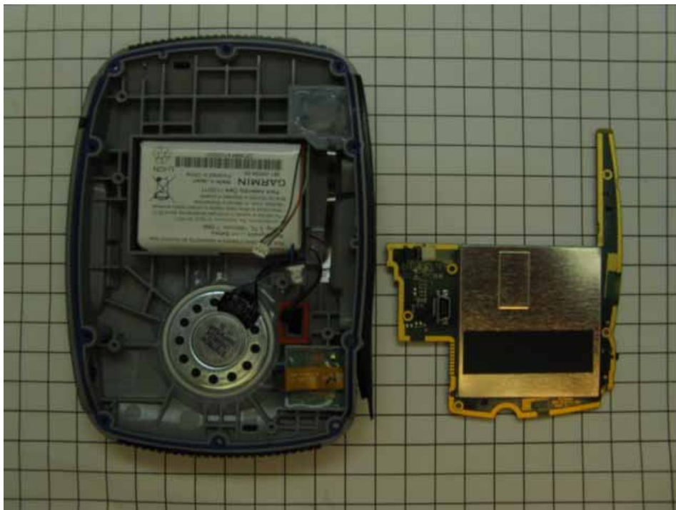
Inside Rear Case and PCB
