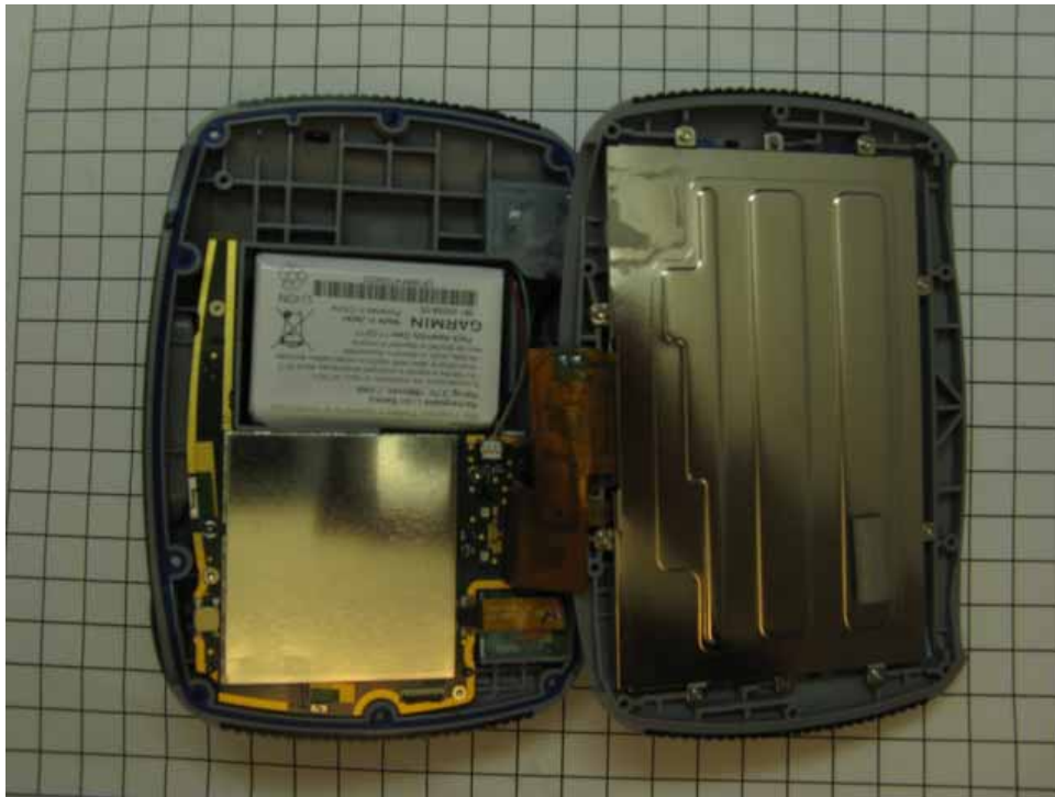
Inside Rear Case and PCB
