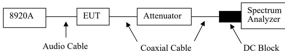
*Note: Path loss from EUT to Spectrum Analyzer is 30.5 dB.*
