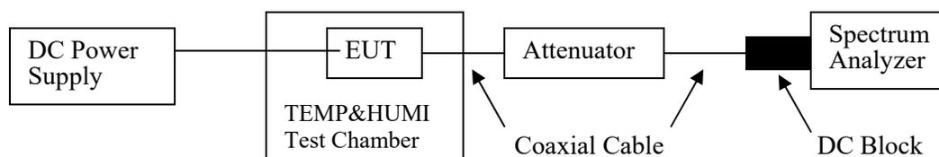
Note: Path loss from EUT to Spectrum Analyzer is 30.5 dB.
