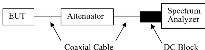
Note: Path loss from EUT to Spectrum Analyzer is 30.5 dB.
