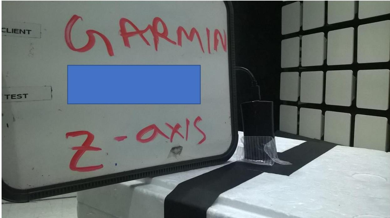
Figure 5 - Radiated Emissions Test Setup, Z-axis
