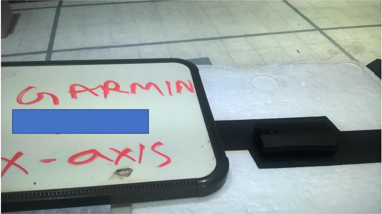
Figure 3 - Radiated Emissions Test Setup, X-axis
