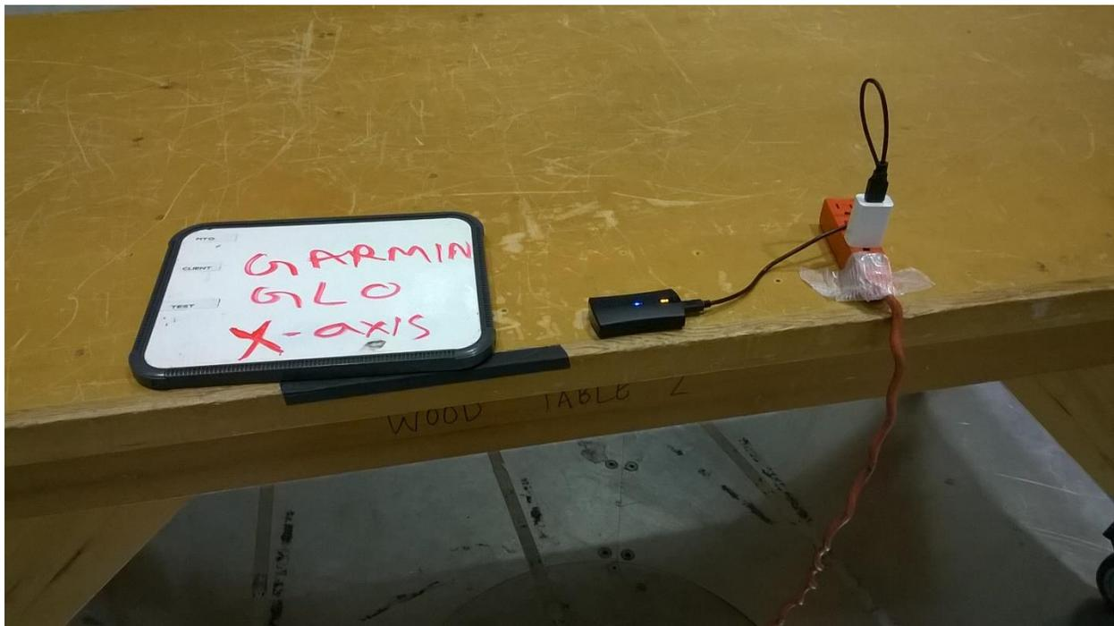
Figure 6 - Radiated Emissions Test Setup, 30MHz - 1GHz
