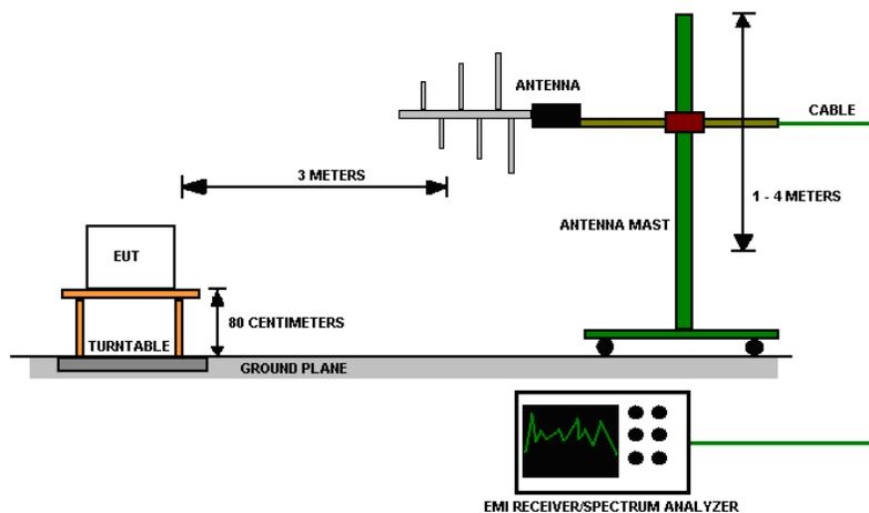
**Figure 1 - Radiated Emissions Test Setup, 30MHz – 1GHz**
