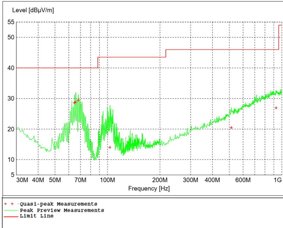
Figure 8 - Radiated Emissions Plot, High Channel
