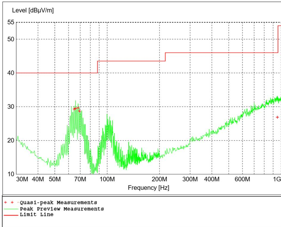
Figure 6 - Radiated Emissions Plot, Low Channel
