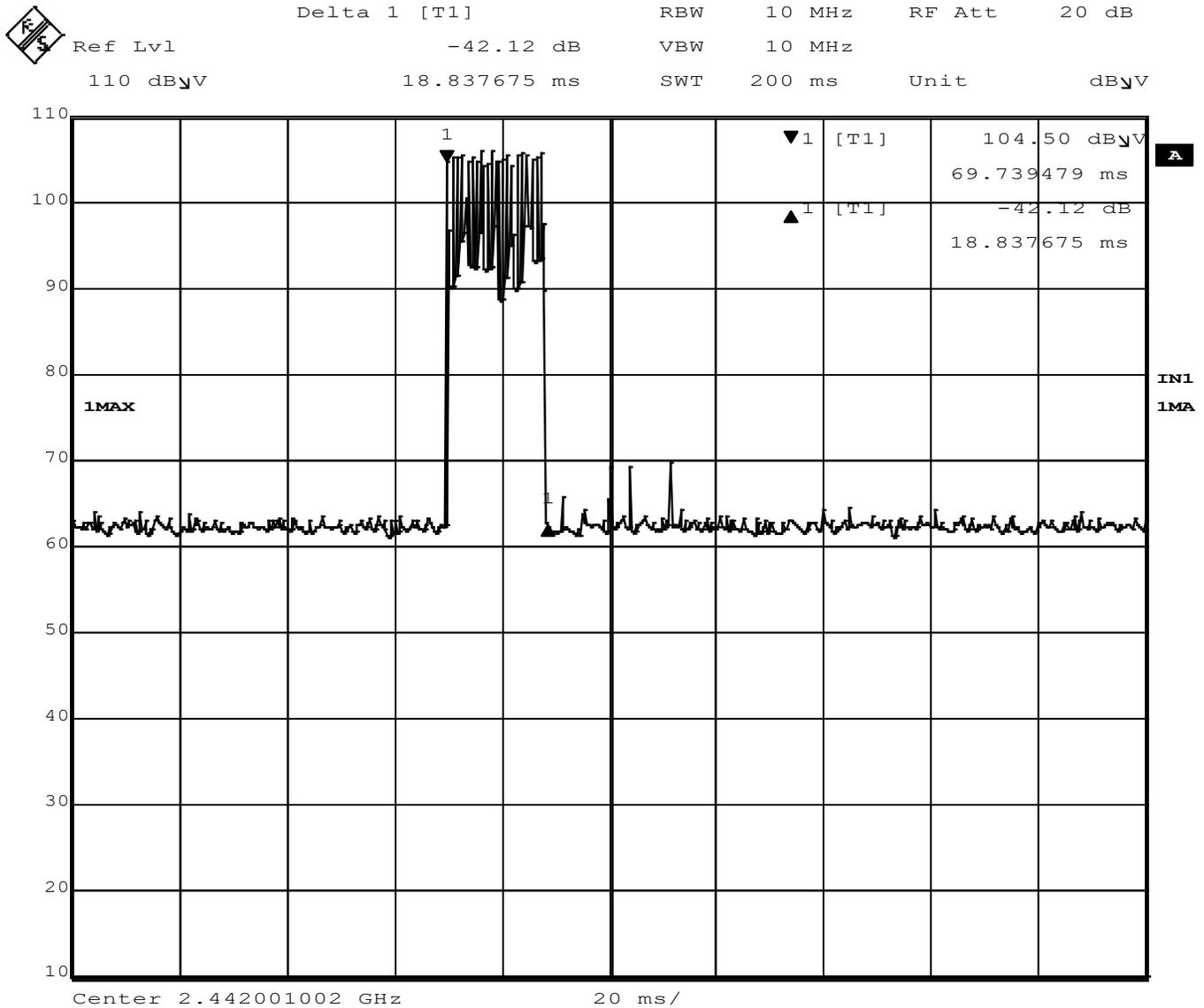
**Figure 3 – Maximum Pulse Width**
