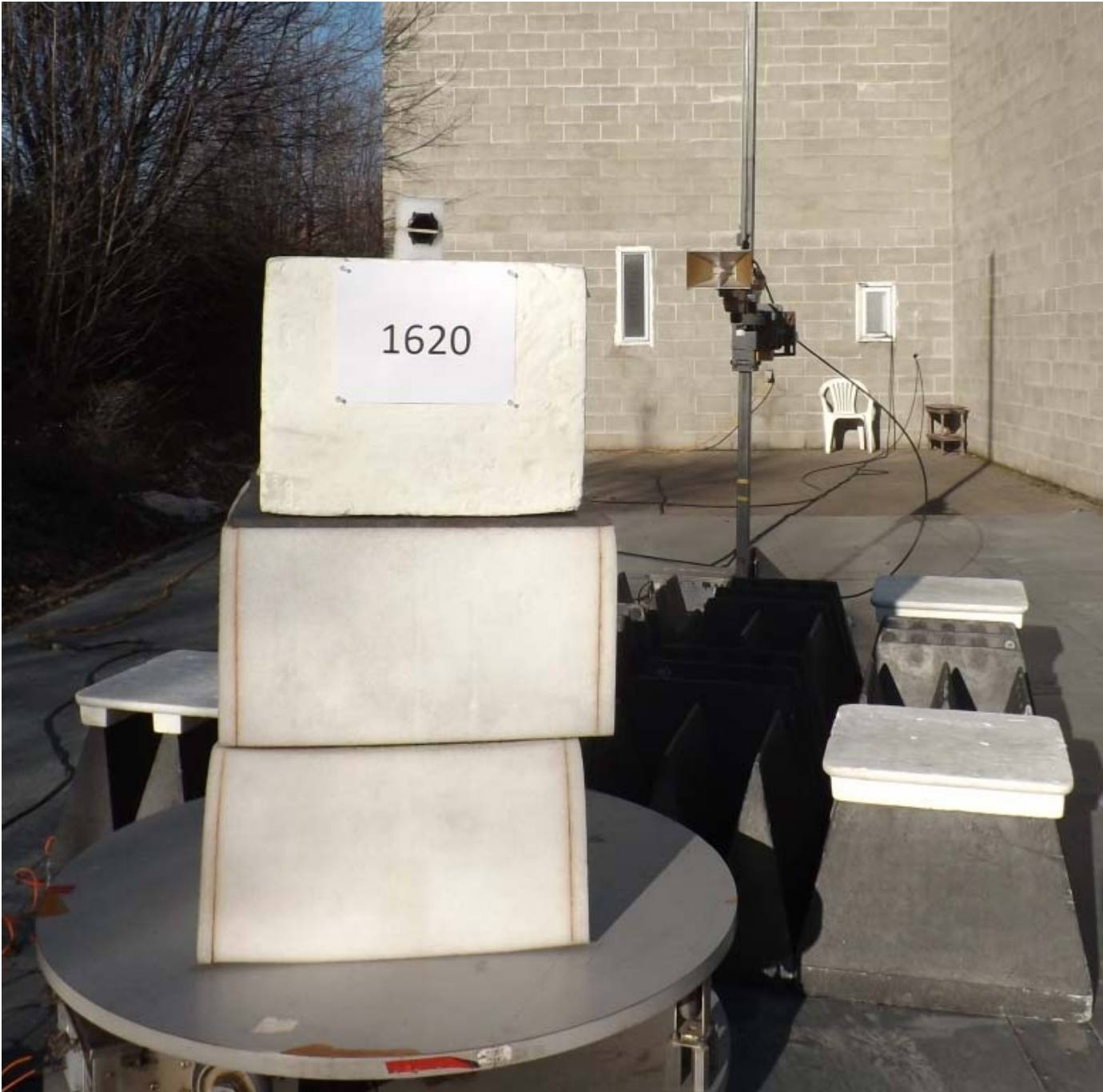
Figure E16.4 – Setup, Radiated Measurements, 1 – 18GHz
