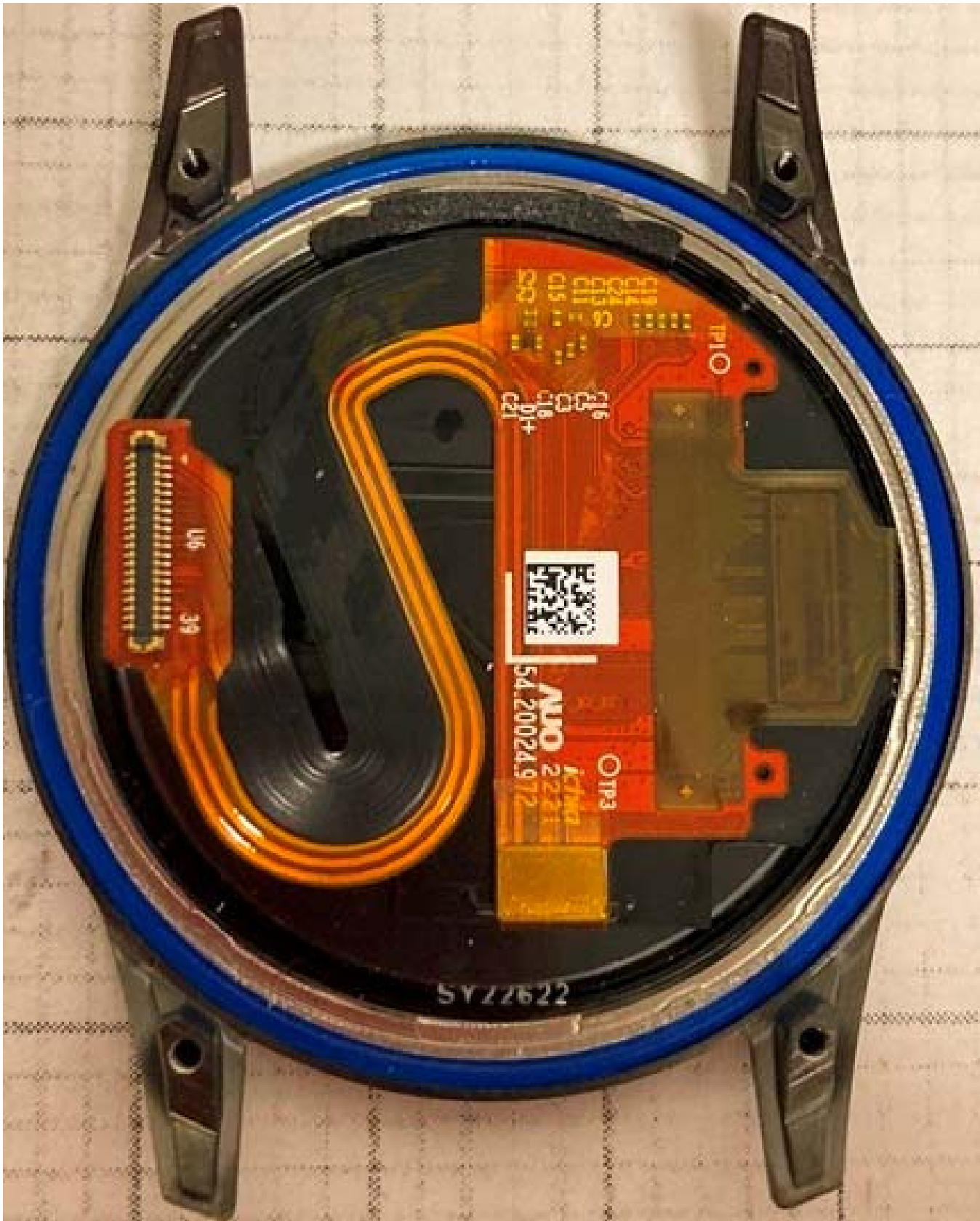
Figure E15.2 – Internal, Front Removed
