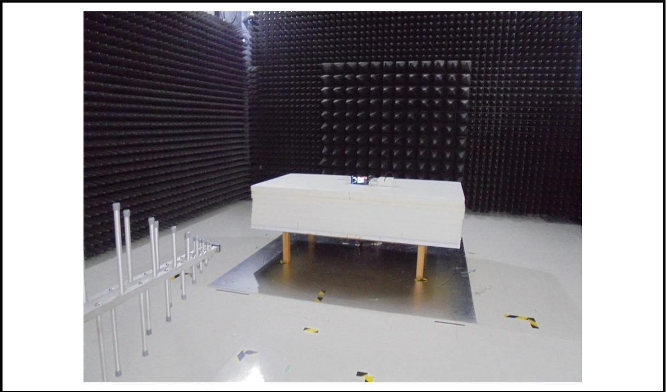
**Radiated Emission Above 1GHz Test**
