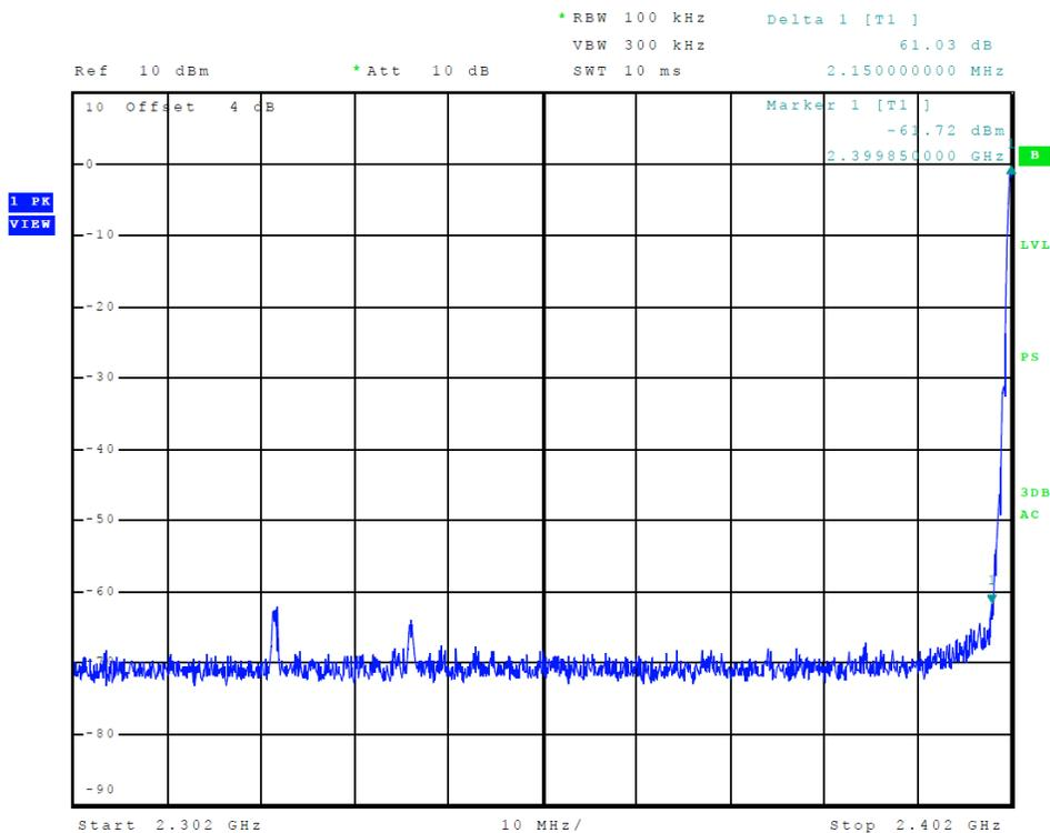
**Figure 4 Plot of Transmitter Emissions (Low Band Edge)**
