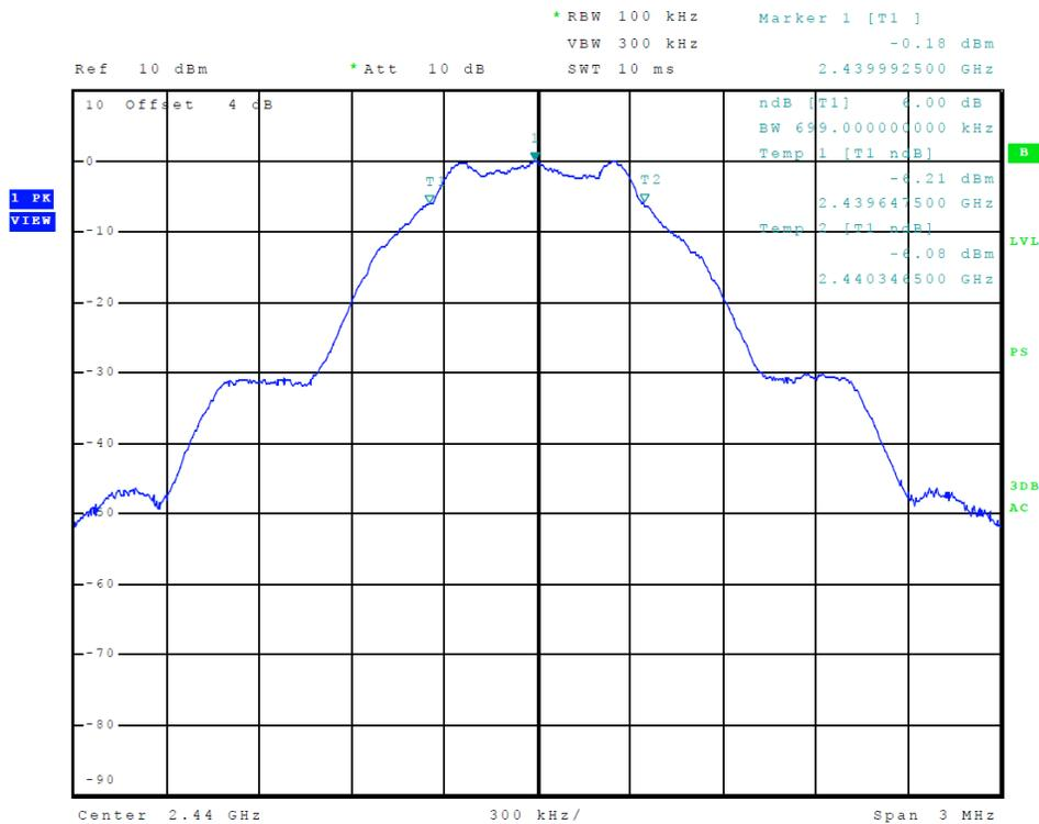
Figure 2 Plot of Transmitter Emissions (6-dB Occupied Bandwidth)
