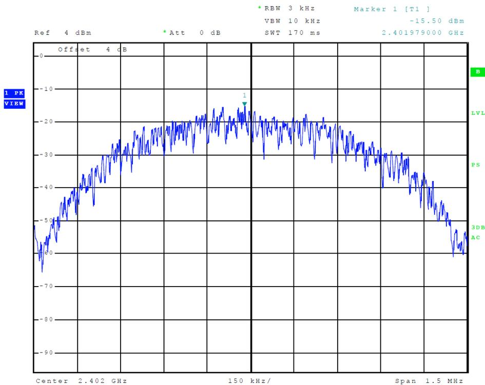
**Figure 6 Plot of Transmitter Emissions (Peak Power Spectral Density)**
