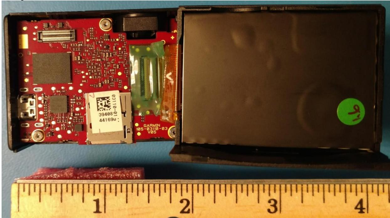
Sensor Board with antenna identification
