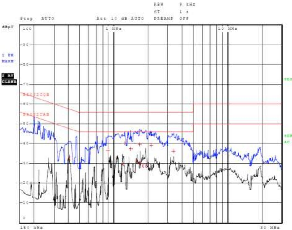
**Figure 5 AC Line Conducted emissions of EUT line 1 (#3, EUT (21) AC Adapter)**
