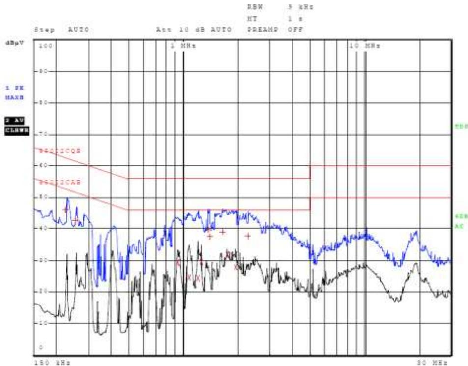
Figure 4 AC Line Conducted emissions of EUT line 2 (#3, EUT (14) AC Adapter)
