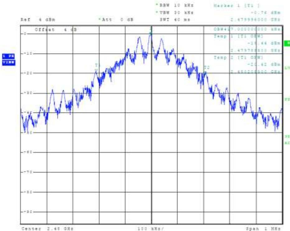
Figure 12 Plot of Transmitter Emissions (Mode 2 99% Occupied Bandwidth)
