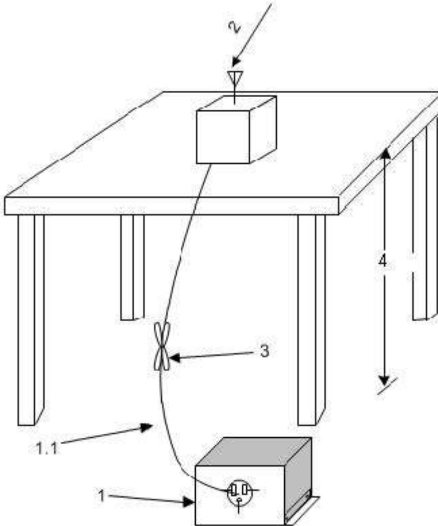
1—A LISN is optional for radiated measurements between 30 MHz and 1000 MHz but not allowed for measurements below 30 MHz and above 1000 MHz (see 6.3.1). If used, then connect EUT to one LISN. Unused LISN measuring port connectors shall be terminated in 50  $\Omega$  loads. The LISN may be placed on top of, or immediately beneath, the reference ground plane (see 6.2.2 and 6.2.3.2).
