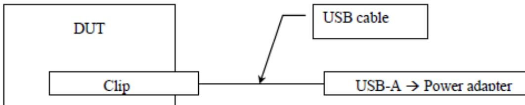
4. DUT transmitting data through wireless 2.4 GHz communication (see test procedure document) and powered by internal battery.
