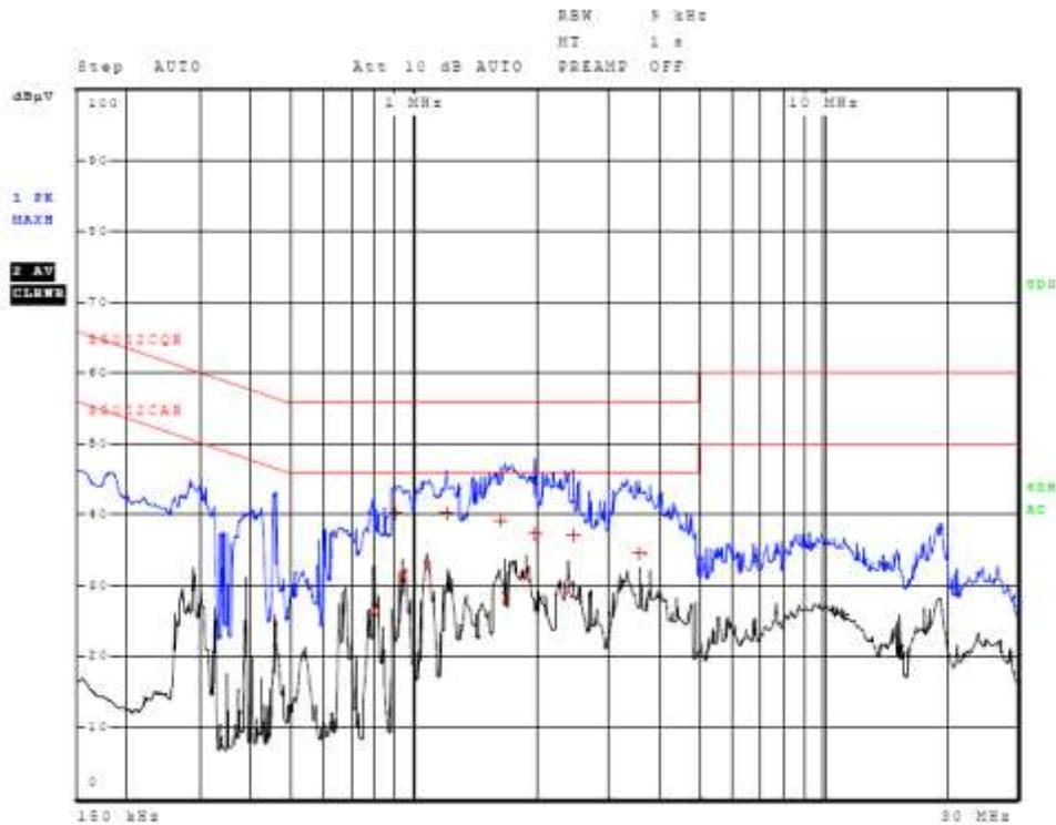
Figure 3 AC Line Conducted emissions of EUT line 1 (#3, EUT (14) AC Adapter)
