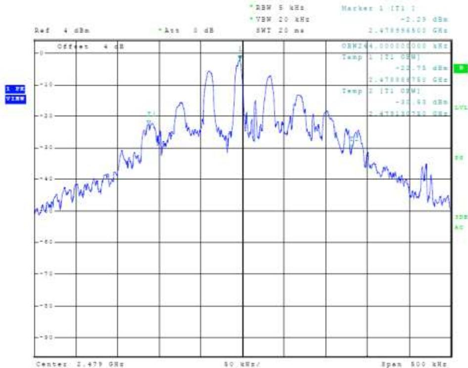
Figure 8 Plot of Transmitter Emissions (Mode 1 99% Occupied Bandwidth)
