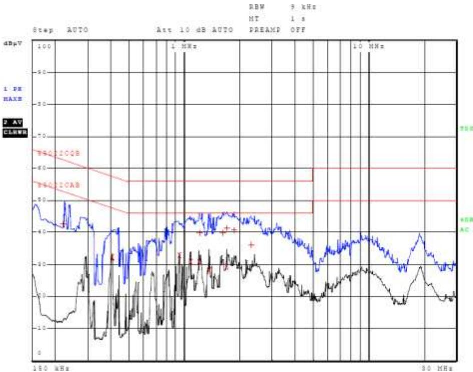
**Figure 6 AC Line Conducted emissions of EUT line 2 (#3, EUT (21) AC Adapter)**
