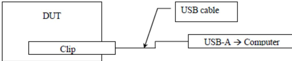
3. DUT internal battery charged by AC or DC power adapter through GPN: 320-01048-00 USB CHARGE CABLE/clip.
