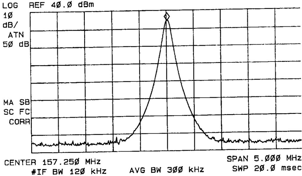
Figure 5: High Power Output Channel 25
