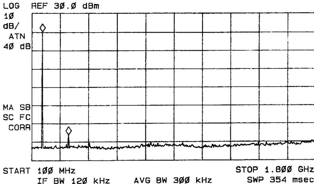
Figure 11: Emissions at Antenna Terminal.
