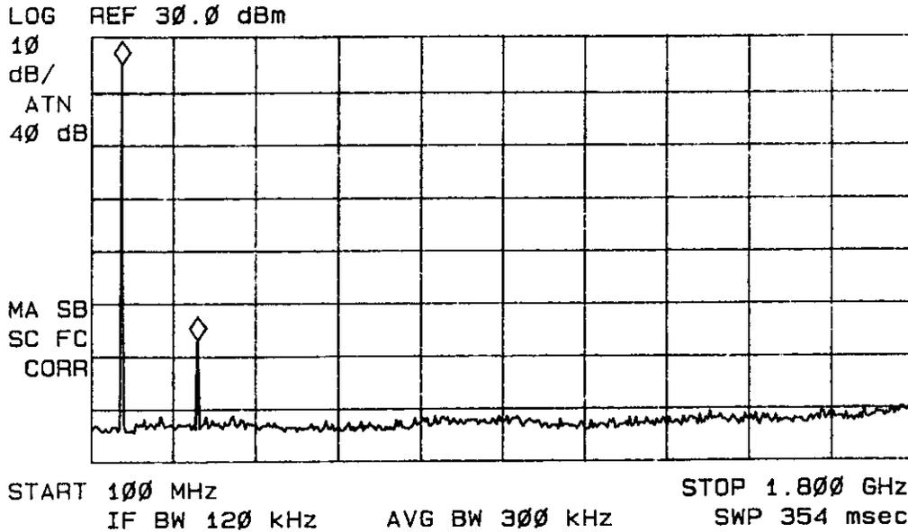
Figure 12: Emissions at Antenna Terminal.
