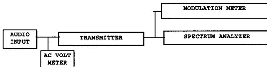
The r.f. output was coupled to a HP Spectrum Analyzer and a modulation meter. The spectrum analyzer was used to observe the r.f. spectrum with the transmitter operating in its various modes. The modulation meter was used to measure the frequency deviation.
