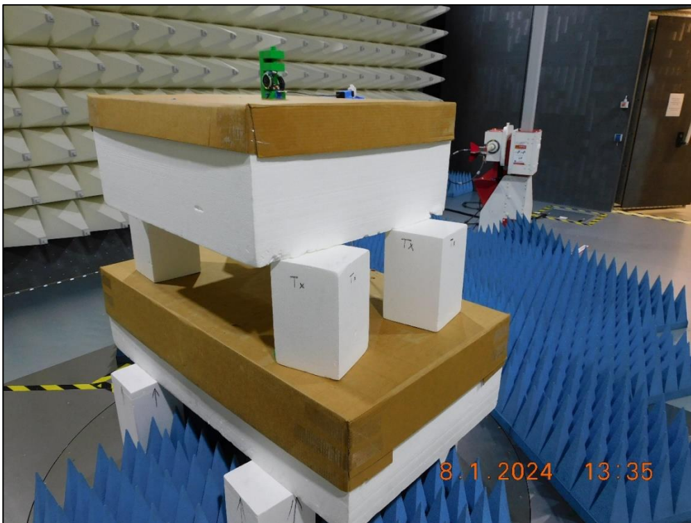
Figure RE21.5: EUT test setup, second view (X orientation Rear view)
